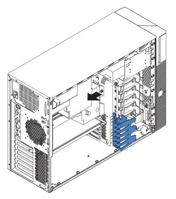
2. Slide the air baffle back slightly and lift it to remove it.
