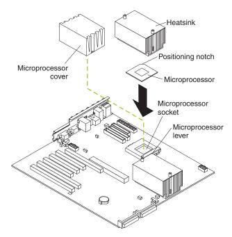
16. When you tighten the screws to secure the heatsink, alternate between the two screws. That is, tighten one screw a little then tighten the other screw a little. Continue switching between the screws until the heatsink is secured to the microprocessor. Alternating the tightening of the screws can help prevent damage to the microprocessor.
