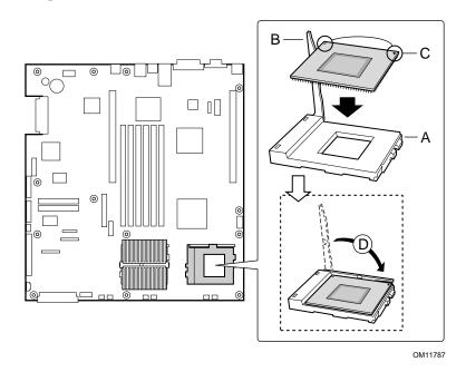
Figure 22. Installing a Terminator
