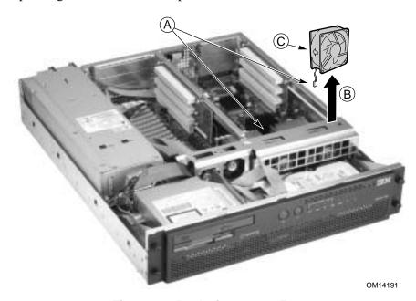
Figure 31. Replacing 80 mm Fans
