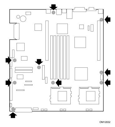
Figure 27. Removing the Server Board Retaining Screws
