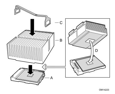
Figure 19. Aligning the Heatsink and Installing the Heatsink Retaining Clip
