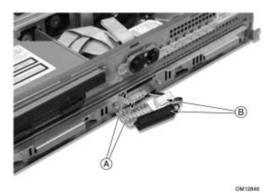
Figure 12. Disconnecting the Hard Disk Drive Bay Cables
