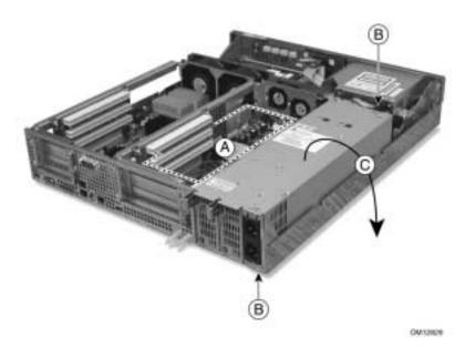
Figure 24. PCI Adapter Cable Installation
