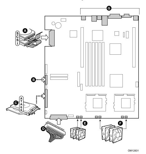
Figure 26. Removing the Server Board Cabling
