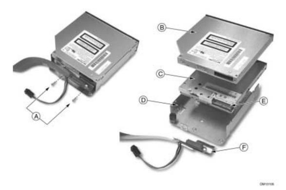
Figure 29. Separating the CD-ROM and Floppy Disk Drives from the Peripheral Bay
