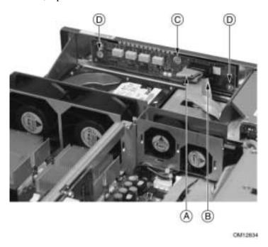
Figure 30. Front Panel Removal
