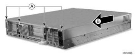
Figure 14. Removing the Top Cover
