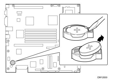
Figure 25. Replacing the Backup Battery
