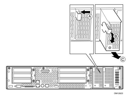
Figure 11. Unlocking and Removing the Power Supply Modules
