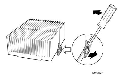
Figure 20. Unlatching the Heatsink Retaining Clip
