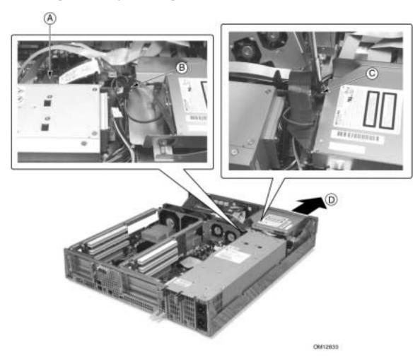
Figure 28. Removing the Peripheral Bay from the Chassis
