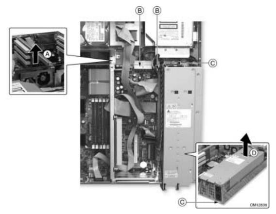
Figure 33. Removing the Power Supply Cage
