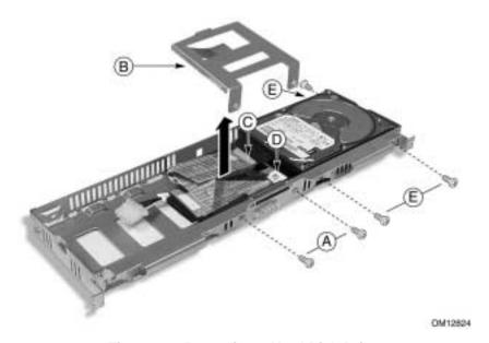
Figure 13. Removing a Hard Disk Drive
