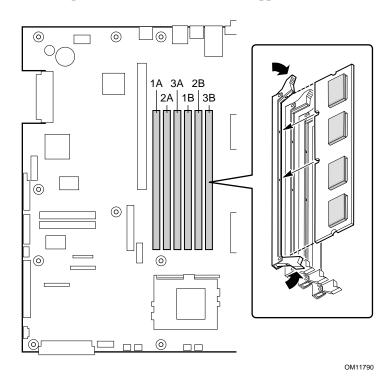
Figure 16. Installing DIMMs
