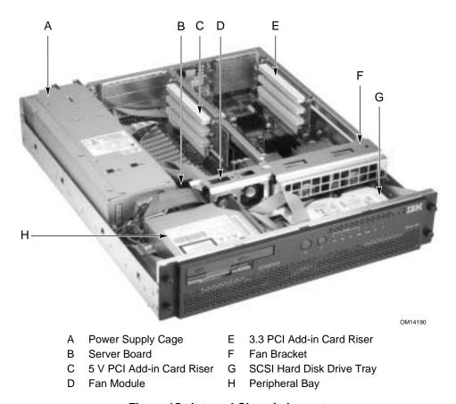
Figure 15. Internal Chassis Layout
