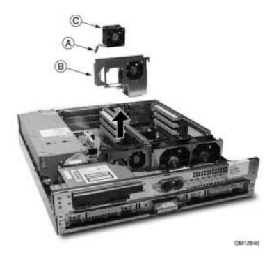
Figure 32. Replacing 40 mm Fans
