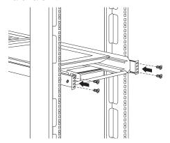
13. While one person pulls the tray halfway out of the front of the rack cabinet and supports the weight of the tray, attach the front of the tray to the rack cabinet using four of the screws from the miscellaneous hardware kit.
