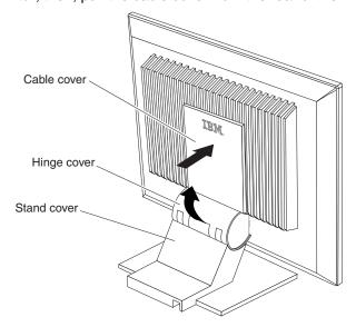
**Note:** Even though the hinge cover and cable cover are not used on the monitor and keyboard tray assembly, do not discard these parts. Store them with the other monitor stand parts you remove for possible future use.
