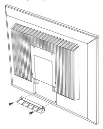
10. Connect the video and power connectors that you disconnected in step 4 on page 13 to the new monitor; then, attach the new monitor to the tray using the four screws that you removed earlier.
