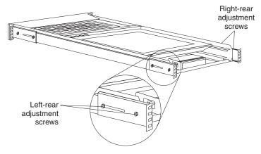
9. Tighten all four slide-rail adjustment screws.
