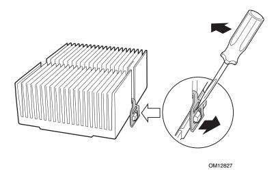
Figure 20. Unlatching the Heatsink Retaining Clip
