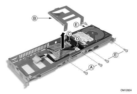
Figure 13. Removing a Hard Disk Drive
