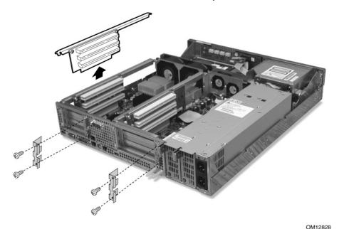
Figure 23. Replacing 3.3 Volt or 5 Volt PCI Add-in Cards
