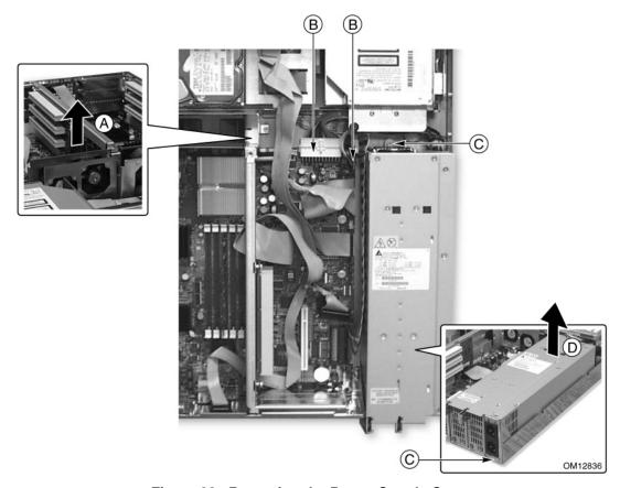
Figure 33. Removing the Power Supply Cage
