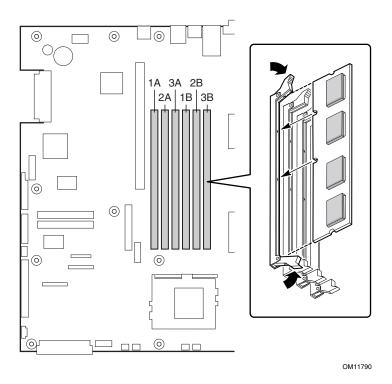
Figure 16. Installing DIMMs
