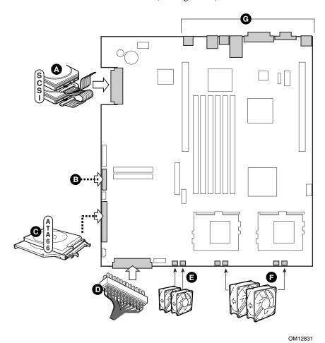
Figure 26. Removing the Server Board Cabling
