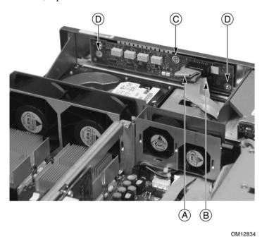
Figure 30. Front Panel Removal
