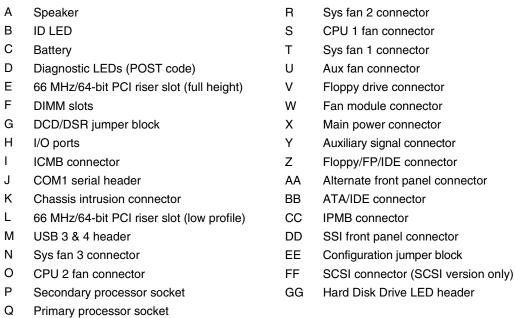
Figure 5. Server Board Connector and Component Locations
