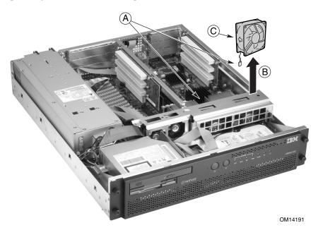
Figure 31. Replacing 80 mm Fans
