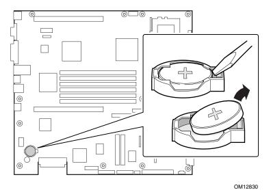
Figure 25. Replacing the Backup Battery
