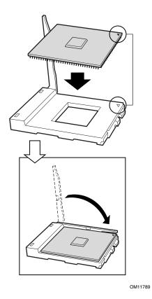
Figure 18. Inserting the Processor and Lowering the Locking Bar
