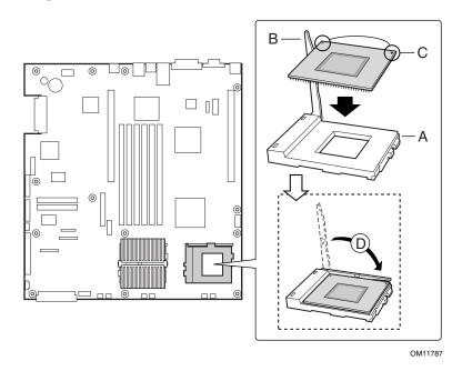
Figure 22. Installing a Terminator
