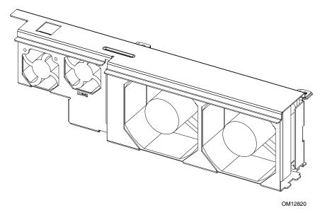
Figure 9. Fan Array with Four System Fans Installed
