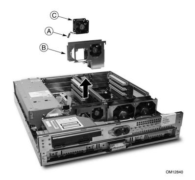
Figure 32. Replacing 40 mm Fans
