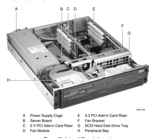
Figure 15. Internal Chassis Layout
