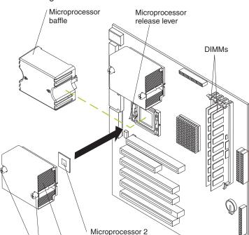
The following illustration shows how to install an additional microprocessor.
