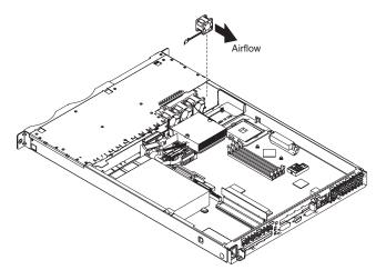
6. Position the replacement fan so that the airflow arrow on the side of the fan is facing or pointing toward the rear of the server.
