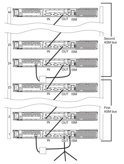
Complete the following steps to cable an ASM interconnect network:
