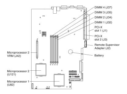
Note: The VRM for microprocessor 1 is integrated into the system board.
