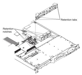
7. Gently pull up on the backplane until it is released from the server at the notches; then, pull the backplane out of the server.
