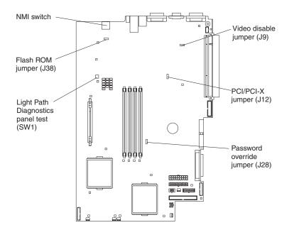
**Note:** The PCI/PCI-X jumper (J12) is used to manually switch PCI-X slot 1 between PCI-X bus B and PCI bus C.
