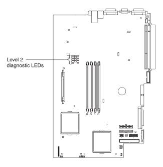
The following illustration shows the error LEDs, light path button, and test LED on Light Path Diagnostics panel on the system board. See "Light Path Diagnostic panel system error LED" on page 82 for information on identifying problems using these LEDs.
