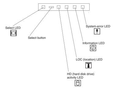
**System-error LED:** When this LED is lit, it indicates that a system error has occurred. A system-error LED is also on the rear of the server. An LED on the Light Path Diagnostics panel on the system board is also lit to help isolate the error.
