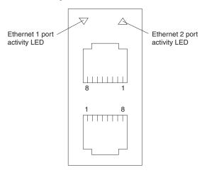
Connect a Category 3, 4, or 5 unshielded twisted-pair cable to this connector. The 100BASE-TX and 1000BASE-T Fast Ethernet standards require Category 5 or higher cabling.
