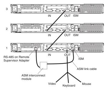
You can add up to 23 more servers to the network by installing a Remote Supervisor adapter in the 24th server, creating a second ASM bus. The following illustration shows an ASM interconnect network with 46 servers.
