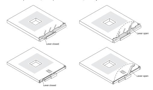
**Note:** The microprocessor-release lever is on the side of the socket that faces the rear of the server.
