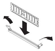
6. Open the retention latches and insert the DIMM straight into the slot, pressing down on both corners of the DIMM at the same time. The side of the DIMM with the gold-edge connectors has an index slot, offset from the center of the DIMM. Align the index slot with the slot on the system board. Ensure that no gap exists between the DIMM and the retaining clips. If a gap does exist, remove the DIMM; then, reinsert it correctly.
