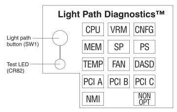
If you remove the server from the rack and you are using the Light Path Diagnostics LEDs to diagnose a problem, you can press the Light Path button to light any LEDs that were lit before you unplugged the server.
