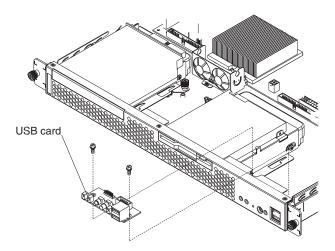
Complete the following steps to remove the Switch/LED/USB card.
