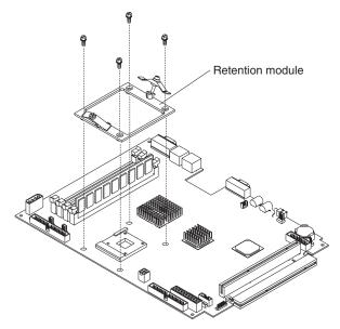
Complete the following steps to remove the retention module.
