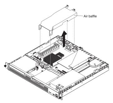
Complete the following steps to remove the air baffle.
