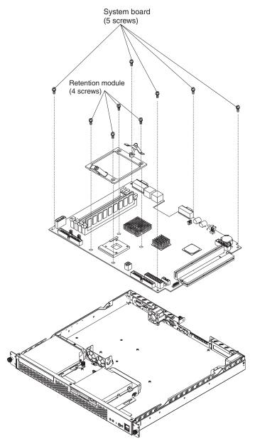
Complete the following steps to remove the system board.
