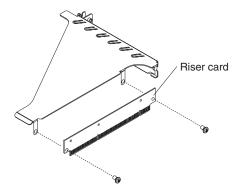
Complete the following steps to remove the PCI riser card.
