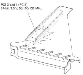
Note: When you install two 133 MHz controllers in the server, the maximum bus speed is 100 MHz.
