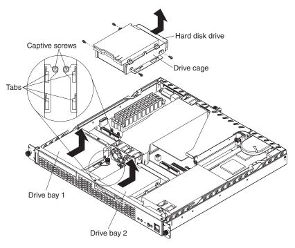
7. Slide the drive cage away from the front of the server until the tabs on the chassis are in the unlocked position. Then, lift the drive cage out of the server.
