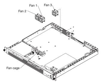
Complete the following steps to remove the fan assembly.
