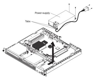
Complete the following steps to remove the power supply.
