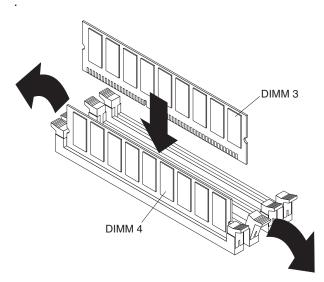
**Attention:** To avoid breaking the retaining clips or damaging the DIMM connectors, open, and close the clips gently.
