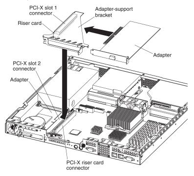
To install the adapter, carefully grasp the adapter by its top edge or upper corners, and align it with the PCI-X expansion slot; then, press the adapter firmly into the expansion slot.
