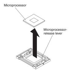
Complete the following steps to remove a microprocessor.
