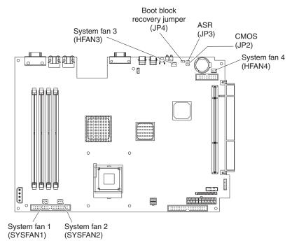
**Note:** The Automatic Server Restart (ASR) jumper (JP3) causes the server to restart automatically if it stops (for example, if the operating system stops running). The default position of the jumper (ASR enabled) is pins 2 and 3.
