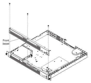
Complete the following steps to remove the front bezel.
