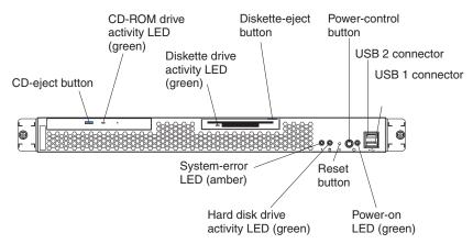
CD-eject button: Press this button to release a CD from the CD-ROM drive.
