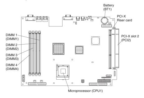
**Note:** Depending on the server model, the server might come with a SCSI adapter installed in PCI-X slot 2.
