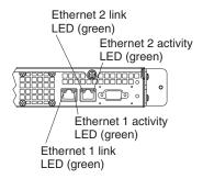
**Ethernet 2 link LED (green):** When this green LED is lit, it indicates that the speed of the Ethernet LAN is 1000BASE-T. When this green LED is off, it indicates that the speed of the Ethernet LAN is 10/100BASE-T.
