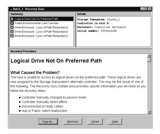
In the Recovery Guru window, the message Logical drive not on preferred path does not necessarily pertain to the current problem. The drive could have been moved to the other controller and not moved back. The loss of redundancy and the failed ESM are what is important.
