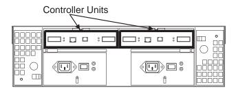
The following figure shows a configuration containing both controllers. It uses GBICs for the connection but does not have the mini hub feature of the 3552. There is a place
