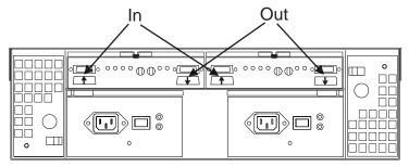
**Note:** In the previous figure, the connections for the GBICs are labeled as In and Out. This designation of the connections is for cabling routing purposes only, as all Fibre cables have both a transmit fiber and receive fiber in them. Any connection can function as either output or input (transmitter or receiver).
