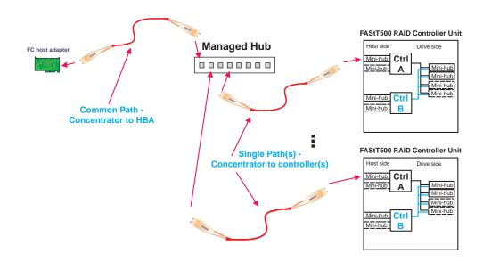
You can also use SANavigator to identify and isolate Fibre Path and device problems. SANavigator discovery for a configuration without concentrators requires that the HBA API Library be installed on the server where SANavigator is installed and in which the HBAs are located. This is referred to as in-band management.
