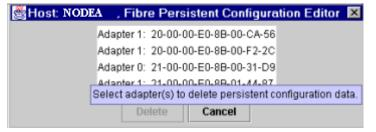
For each adapter connected to the host, the current persistent configuration editor lists the adapter number and its world wide port name.
