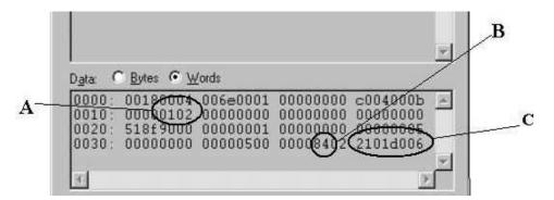
**A.** This error indicates (according to the error codes listed in Table 6) a recovered error.
