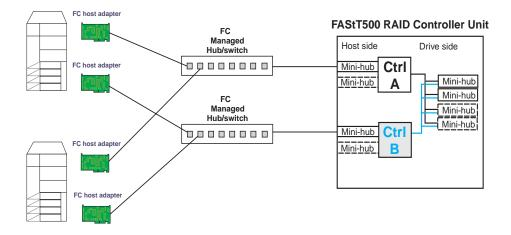
2. All I/O is flowing through controller A. This yields the following diagram for debugging.
