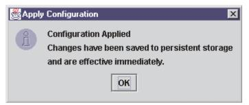
• Click **Save** to save the new configuration. The new configuration is saved to the persistent configuration file; it will be used the next time the system is started. The current configuration remains in memory and is redisplayed after the save operation completes.
