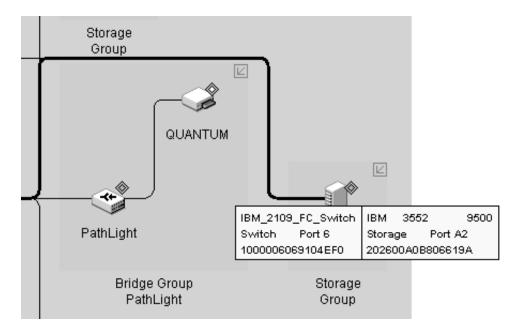
• Expand multi-port devices to show the port assignments. Right-click the device and select **Ports** from the pop-up menu to view the ports.
