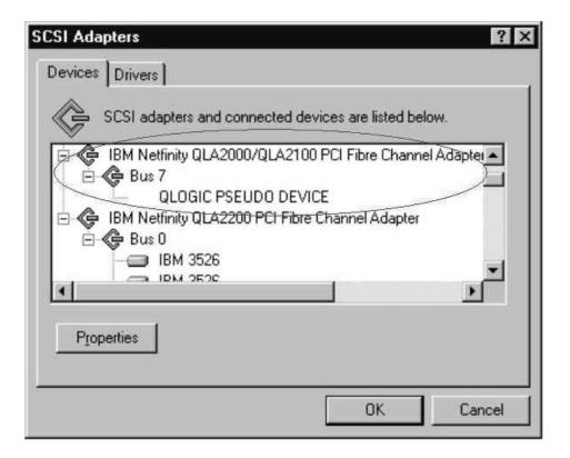
There are no other devices; there should have been a Bus 0 with 21 of the IBM 3526s and one IBM Universal Xport. Note the 2100 DD shows up as started in the Drivers tab here and in the Control Panel Devices applet.
