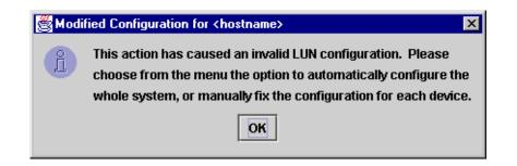
This problem is usually the result of changing the configuration state of a device. You must modify the LUN configuration for this device before you can save or apply the configuration.
