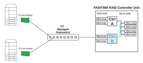
3. To see more clearly what is involved, redraw the configuration showing the path elements in the loop, as in the following figure.
