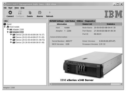
A different configuration is shown in the following figure, which shows a 2200 adapter. Its World Wide Name is 20-00-00-E0-8B-A1-30 and it has five devices
