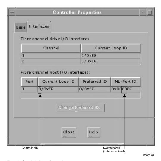
Figure 8. Controller Properties window
