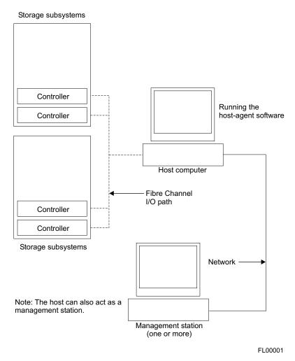
Figure 1. Host-agent (in-band) managed storage subsystems
