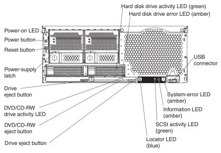
**Power-on LED:** This green LED turns on and stays on when you turn on your server, and it flashes when the server is in Standby mode.
