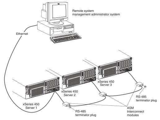
**Note:** The ASM Interconnect module is connected to the RS485 port on the back panel of the Remote Supervisor Adapter in each server.
