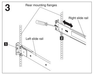
Use the tab **1** on the rear of each slide rail to align the slide rail to the rear mounting flanges. If the front slide rail bracket does not align with the front mounting flange, slightly loosen the rail-length-adjusting screws **2** and adjust the length of the rail.
