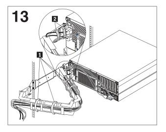
Route the cables through the cable-management arm, securing them with cable straps **1**. Use two cable straps **2** (one on each side of the hinge) to secure the power cords to the hinge plate.
