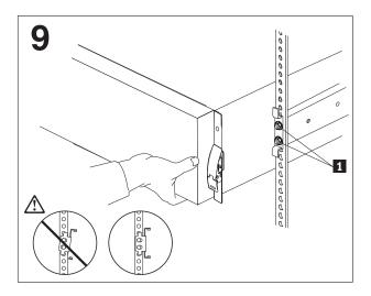
Slide the server halfway out of the rack cabinet; then, loosen but do not remove the four front M6 screws 1. While one person supports the front of the server by lifting it slightly, ensure that the front slide-rail brackets are vertically aligned; then, fully tighten the four front M6 screws.
