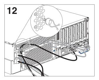
Attach the cables to the rear of the server (including keyboard, mouse, and monitor cables if required). Route the cables to the left side of the server. Use cable clamps to secure the cables. Insert clamps only in the column of ventilation holes immediately to the right of the ac power connectors. If you insert the clamps in columns elsewhere, they will interfere with the removal of internal components.
