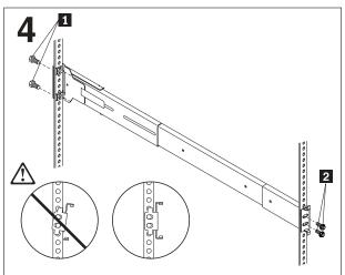
Install the slide rails, ensuring that the front and rear slide rail brackets for both slide rails are vertically aligned. Insert and partially tighten the four rear M6 screws 1; then, insert and fully tighten the four front M6 screws 2.
