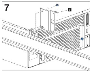
Insert the tab on the bottom edge of the cable management arm hinge plate **1** into the slot at the rear of the server; then, attach the plate to the server with the M3.5 thumbscrew.
