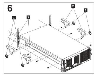
Use four M4 screws per side to secure the server to the rails; then, remove the rack-support wheels 1 and the handles 2 and store them in a safe place.
