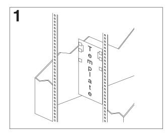
Use the attached stickers to mark the holes on the front and rear rack cabinet mounting flanges as indicated by the arrows on the attached rack mounting template.
