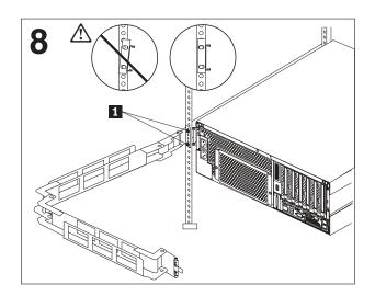
Press in on the slide-rail locking latches and slide the server fully into the rack cabinet. Slide the cable-management-arm bracket over the M6 screws **1**. Ensure that both rear slide-rail brackets are vertically aligned; then, fully tighten the four rear M6 screws.
