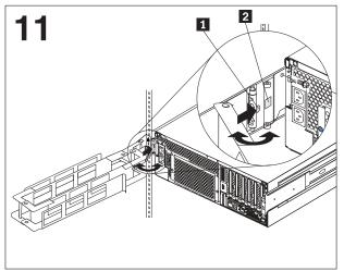
Slide the tab **1** on the cable management arm into the slot **2** in the hinge plate; then, release the hinge pins into the holes in the plate.
