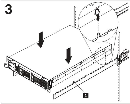
Extend the slide rails fully from the rack until the slide rails lock. Align the tabs on the slide rails **1** with the matching inserts on the server and lower the server on the slide rails.
