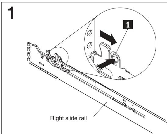
Push outward on the slide-rail latch **1**; then, pull the latch back to open the slide rail. The latch will catch to stay open. Open the other end of the slide rail; then, do the same for the other slide rail.
