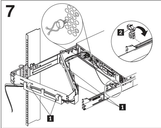
Attach the power cords and other cables to the rear of the server (including keyboard, monitor, and mouse, if required). Attach the power cords to the cable-restraint bracket **2**. Secure the cable-restraint bracket to the slide rail.
