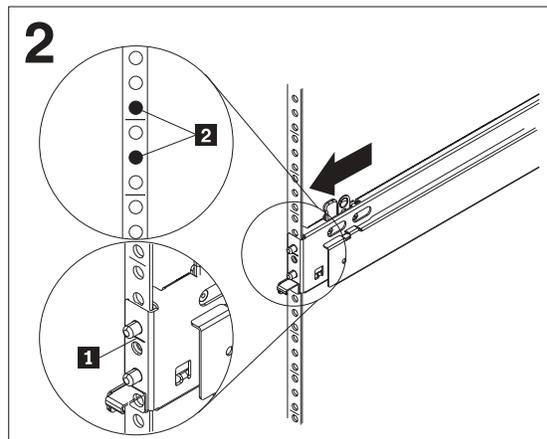
Align the slide rail with the front mounting flange. Use the score mark on the slide rail **1** to align the slide rail. Push outward on the slide-rail latch to close the latch and secure the slide rail. Do the same for the other front slide rail. Align the slide rail with the rear mounting flange. The slide rail occupies the full height of the server. Close the latches to secure the rear of both slide rails.
