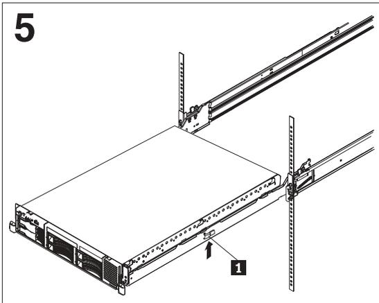
Lift the locking levers **1** on the slide rails and slide the server into the rack until it extends approximately 4 inches.
