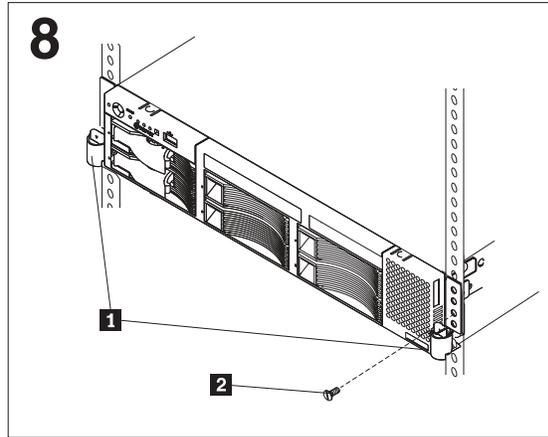
Slide the server into the rack cabinet until the release latches **1** lock into place. To slide the server out of the rack, press on the release latches.
