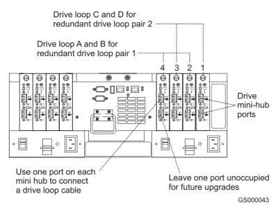
Figure 4. Drive mini-hub ports
