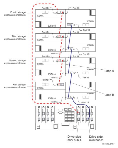
Figure 6. EXP 810 storage expansion enclosure
