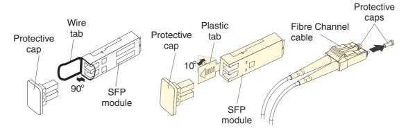
Figure 1. SFP modules and fibre channel cables
