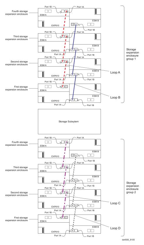
Figure 71. Connecting a second redundant EXP810 storage expansion enclosure group (loops C and D)
