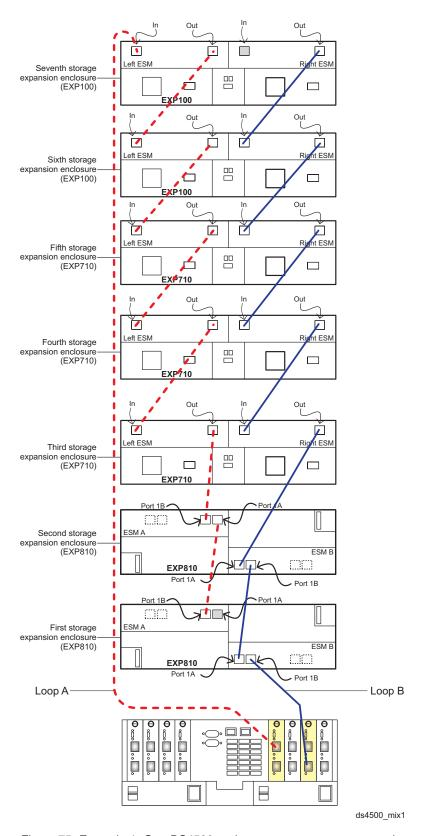
Figure 75. Example 1: One DS4500 and two or more storage expansion enclosures in a mixed environment — Recommended cabling
