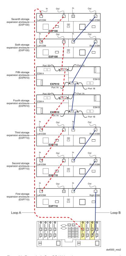
Figure 76. Example 2: One DS4500 and two or more storage expansion enclosures in a mixed environment — Recommended cabling
