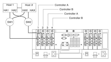
Figure 80. Using two fibre channel switches to connect a host
