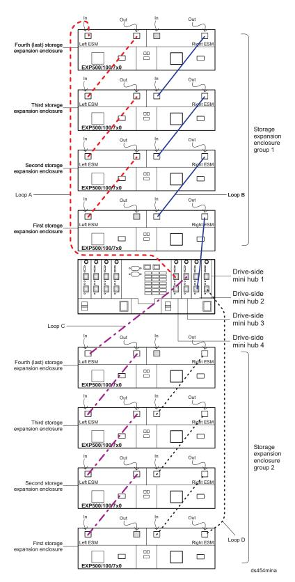
Figure 66. Connecting two redundant EXP500, EXP100, EXP700, or EXP710 storage expansion enclosure groups
