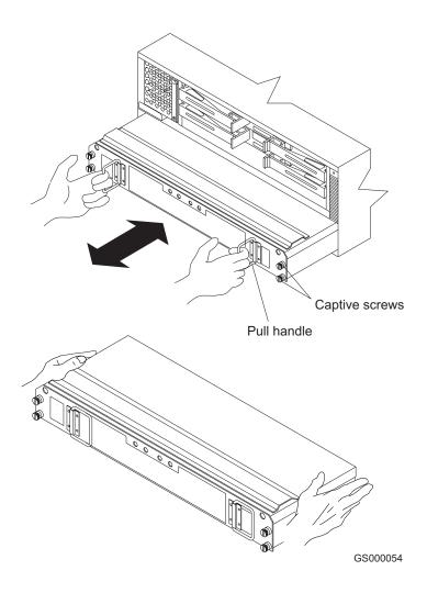
Figure 100. Removing and installing a battery unit
