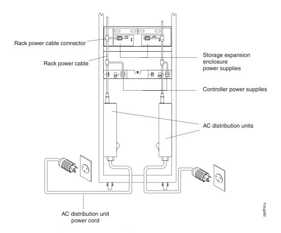
Figure 85. Redundant AC power connections to controllers and storage expansion enclosures
