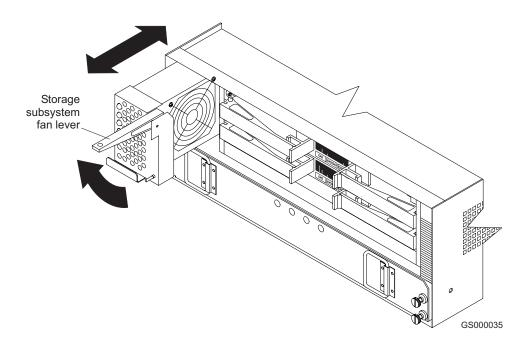
Figure 102. Removing and installing the storage subsystem fan
