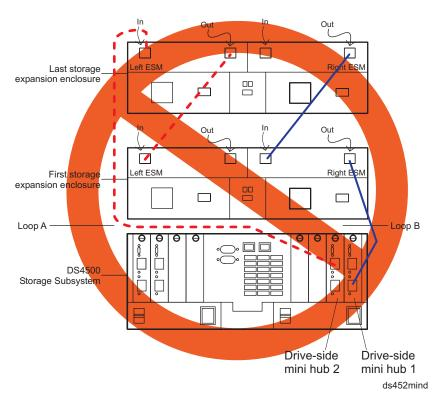
Figure 57. Redundant drive loop cabling overview with two drive mini hubs in slots 1 and 2 - Not for use unless you meet the requirements in the Note above
