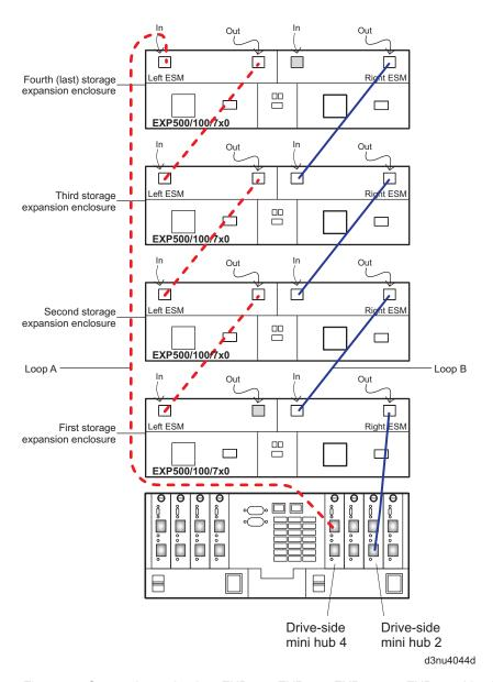
Figure 65. Connecting redundant EXP500, EXP100, EXP700, or EXP710 drive loops to the DS4500
