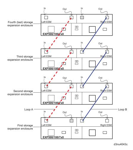
Figure 62. Connecting additional EXP500, EXP100, EXP700, or EXP710 storage expansion enclosures to drive loops A and B
