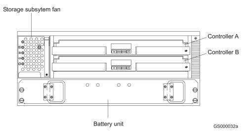
Figure 1. IBM TotalStorage DS4500 Storage Subsystem - front view
