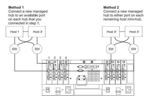
Figure 81. Using four fibre channel switches to connect multiple hosts
