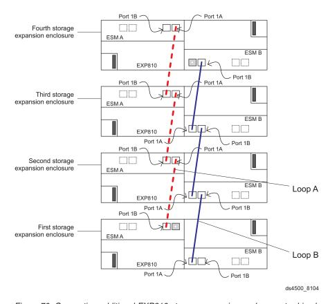
Figure 70. Connecting additional EXP810 storage expansion enclosures to drive loops A and B
