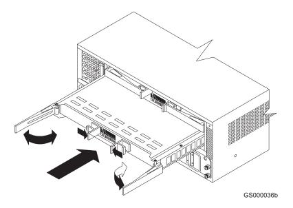
Figure 23. Replacing a controller
