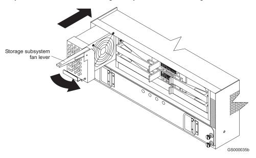
Figure 22. Replacing the storage subsystem fan
