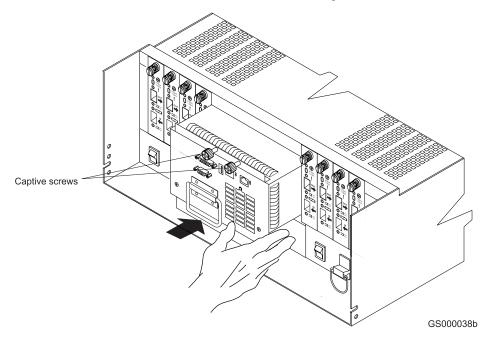
Figure 26. Replacing a fan and communications module
