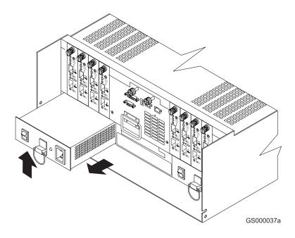
Figure 17. Power supply removal
