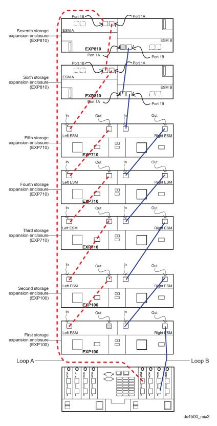
Figure 48. Correct cabling for an intermix of EXP100, EXP710, and EXP810 storage expansion enclosure (example 1)
