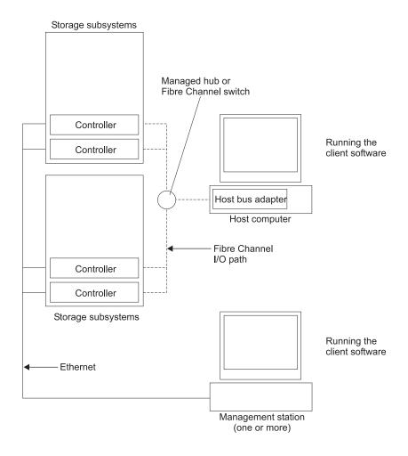
Figure 78. Direct (out-of-band) managed storage subsystems
