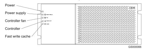
Figure 99. LEDs on the DS4500 Storage Subsystem bezel
