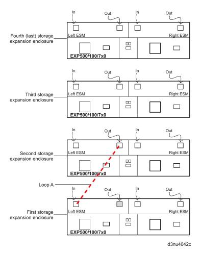
Figure 59. Connecting two EXP500, EXP100, EXP700, or EXP710 storage expansion enclosures into drive loop A
