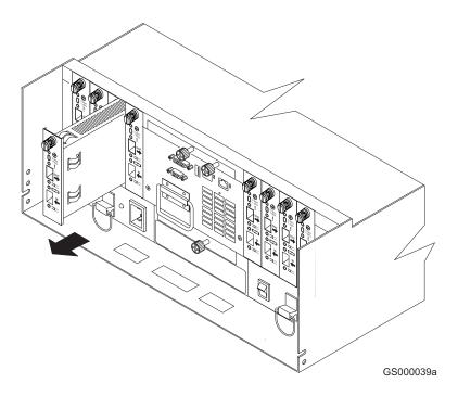
Figure 19. Mini hub removal
