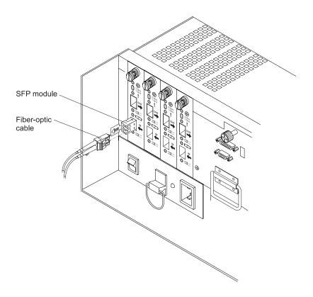
Figure 35. Installing an SFP module into the host port
