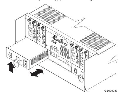
Figure 107. Removing and installing a power supply
