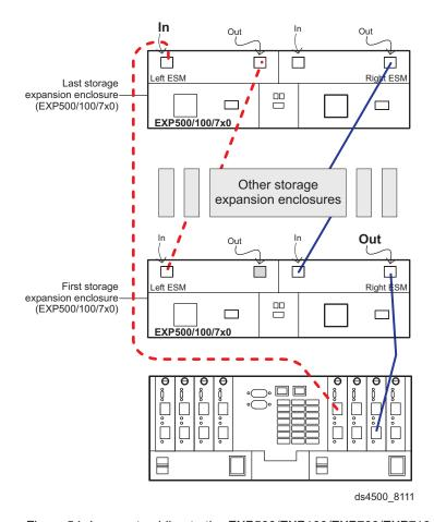
Figure 54. Incorrect cabling to the EXP500/EXP100/EXP700/EXP710 ports
