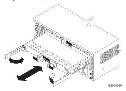
Figure 98. Removing and replacing a failed controller CRU
