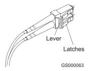
Figure 46. LC-LC fibre-channel cable lever and latches
