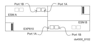
Figure 68. EXP810 storage expansion enclosure ESM board ports 1A and 1B
