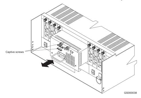
Figure 105. Removing and installing a fan and communications module
