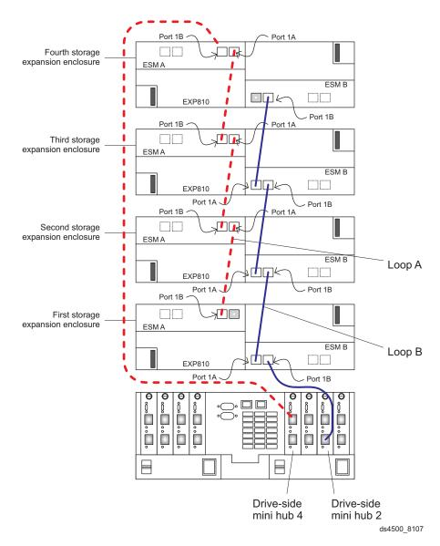
Figure 73. Connecting redundant EXP810 drive loops to the DS4500
