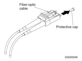
Figure 39. Removing fiber-optic cable protective caps
