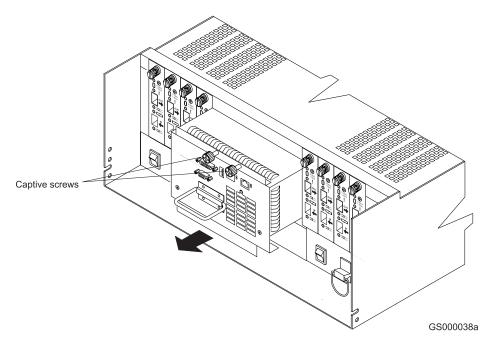
Figure 18. Fan and communications module removal
