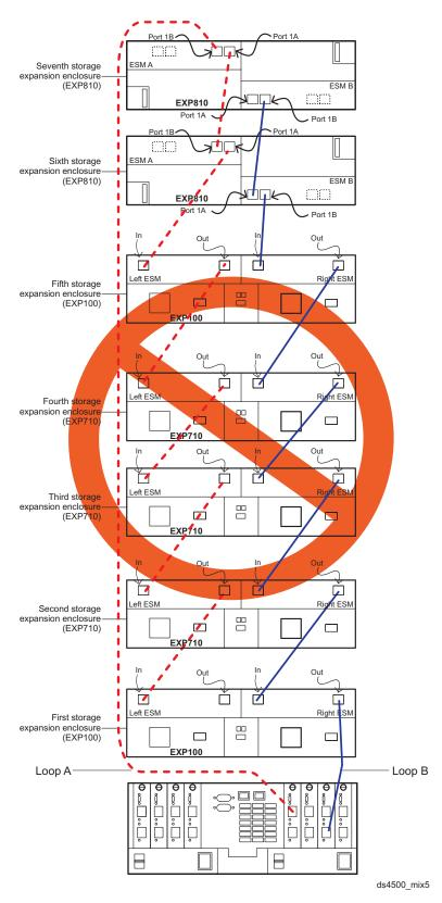
Figure 50. Incorrect cabling for an intermix of EXP100, EXP710, and EXP810 storage expansion enclosure (example 1)
