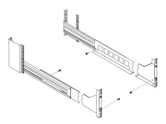
Figure 20. Controller unit screw removal
