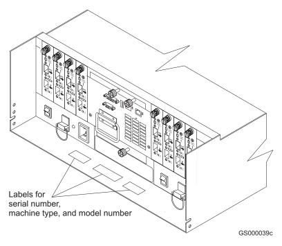
Figure 8. Example of DS4500 serial number, machine type, and model number location
