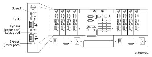
Figure 93. Mini hub LEDs
