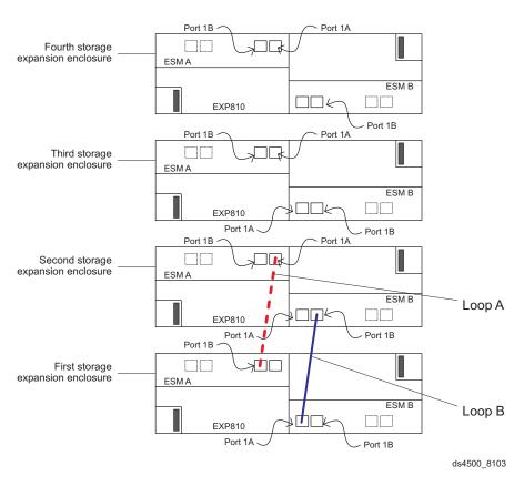
Figure 69. Connecting two EXP810 storage expansion enclosures into redundant drive loop B
