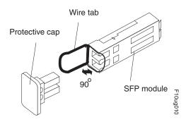
Figure 37. Unlocking the SFP module latch - wire variety
