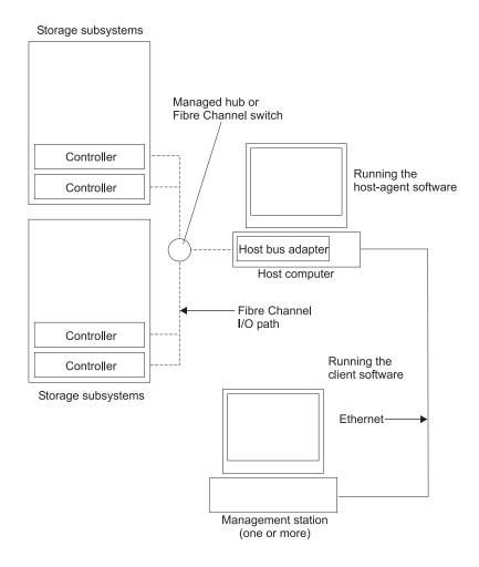
Figure 77. Host-agent (in-band) managed storage subsystems
