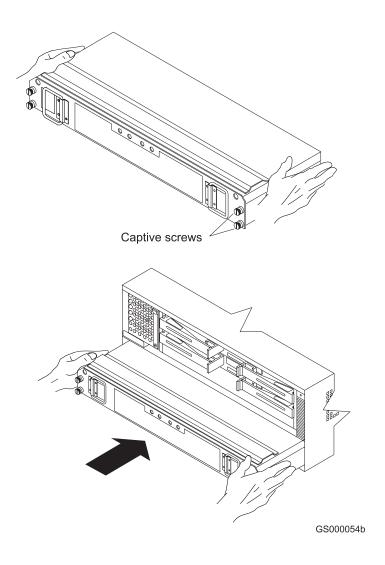
Figure 24. Replacing a battery unit
