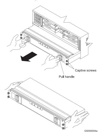
Figure 16. Battery unit removal
