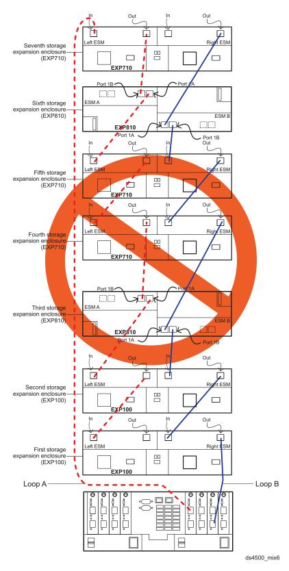
Figure 51. Incorrect cabling for an intermix of EXP100, EXP710, and EXP810 storage expansion enclosure (example 2)
