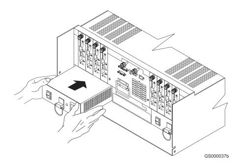
Figure 25. Replacing a power supply
