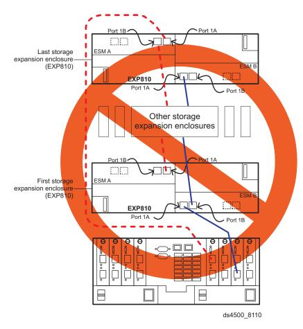
Figure 53. Incorrect cabling to the EXP810 port
