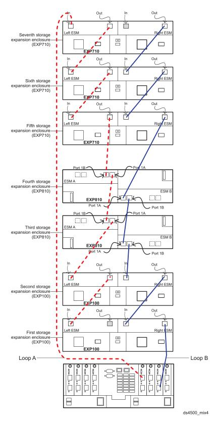
Figure 49. Correct cabling for an intermix of EXP100, EXP710, and EXP810 storage expansion enclosure (example 2)
