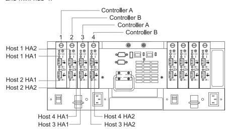
Figure 79. Connecting hosts directly to the controller
