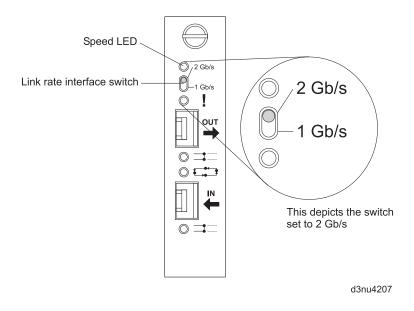
Figure 86. Mini hub Link Rate Interface switch and Speed LED
