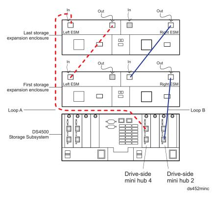
Figure 56. Redundant drive loop cabling overview with two drive mini hubs in slots 4 and 2
