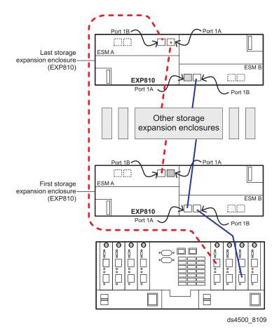
Figure 52. Correct cabling to EXP810 port 1B
