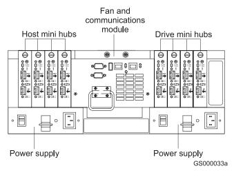
Figure 2. IBM TotalStorage DS4500 Storage Subsystem - back view
