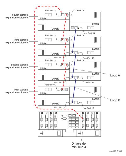
Figure 72. Connecting EXP810 drive loop A to the DS4500
