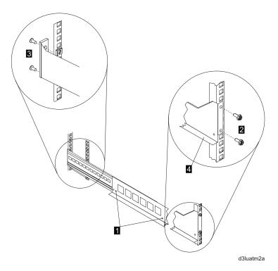
Figure 11. Installing the support rails
