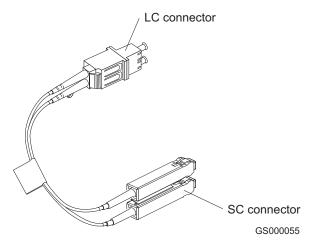
Figure 43. LC-SC fibre-channel cable adapter
