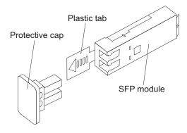
Figure 34. SFP module and protective cap
