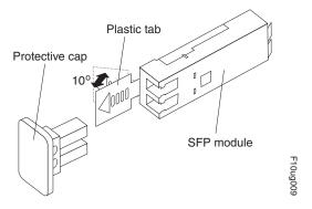
Figure 36. Unlocking the SFP module latch - plastic variety
