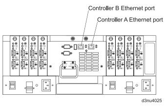
Figure 33. Ethernet ports
