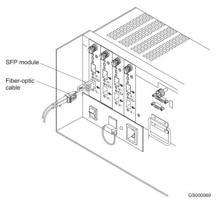
Figure 110. Replacing an SFP module
