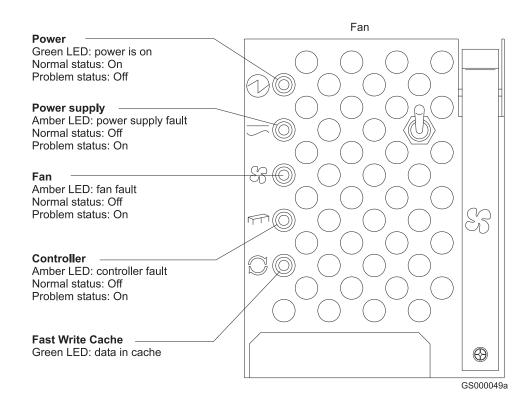
Figure 103. Storage subsystem LEDs
