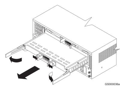
Figure 15. Controller removal
