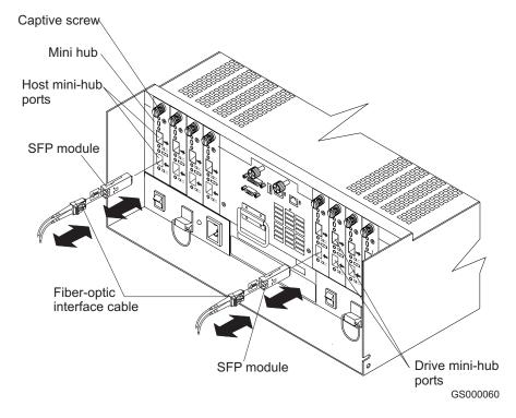
Figure 108. Removing the fiber-optic cable from the SFP module
