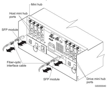
Figure 29. Fibre Channel interface connections
