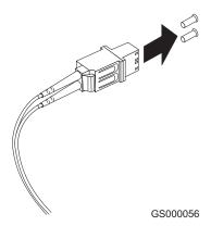
Figure 44. Removing the LC-SC cable adapter protective caps
