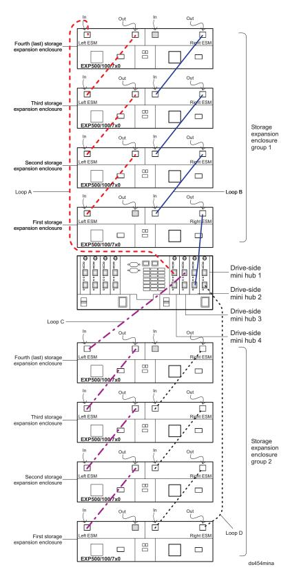
Figure 58. Redundant drive loop cabling overview — four drive mini hubs
