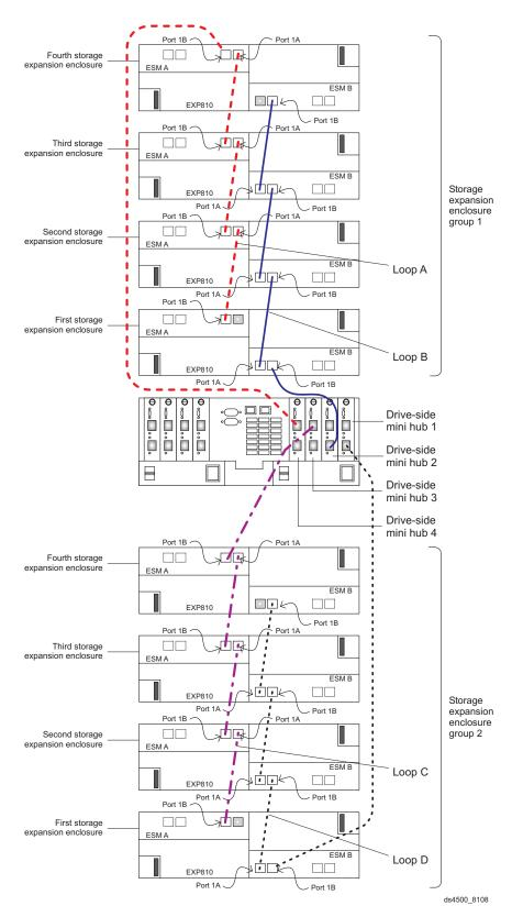
Figure 74. Connecting two redundant EXP810 storage expansion enclosure groups
