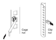
Figure 12. Cage nut and slide clip nut insertion
