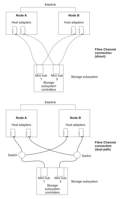
Figure 83. Host adapters in storage subsystems on a fibre channel network
