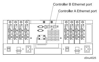
Figure 104. Fan and communications module ports
