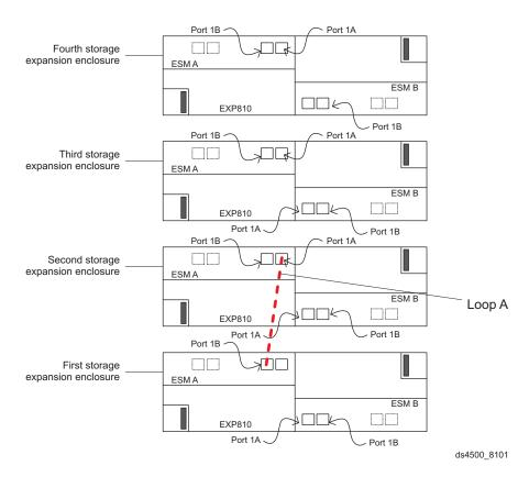
Figure 67. Connecting two EXP810 storage expansion enclosures into drive loop A
