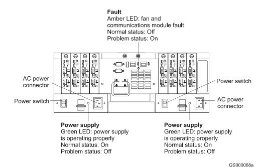
Figure 106. Power supply switch, AC power connectors, and indicator lights
