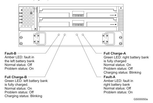
Figure 90. Battery unit LEDs
