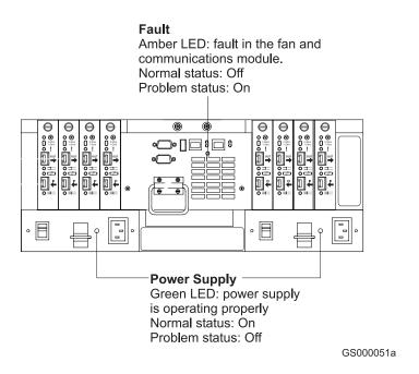
Figure 94. Fan and communications and power supply fault LEDs
