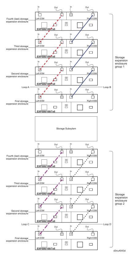
Figure 63. Connecting a second redundant EXP500, EXP100, EXP700, or EXP710 storage expansion enclosure group (loops C and D)
