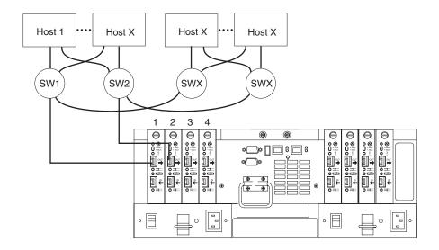
Figure 82. Adding hosts by using cascading switches
