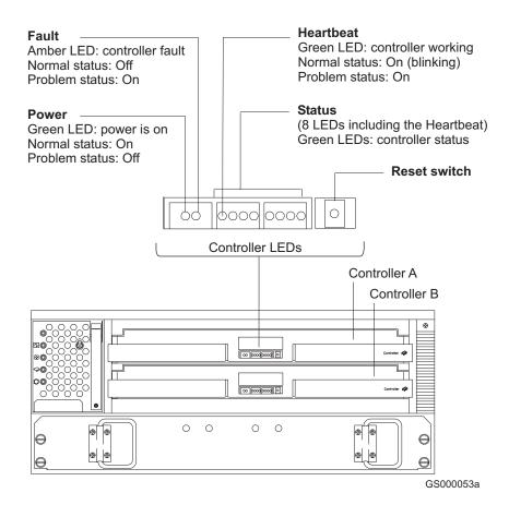
Figure 89. Controller LEDs
