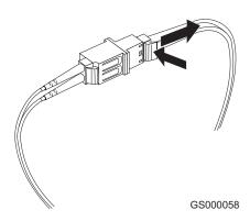
Figure 47. Removing the LC-LC fibre-channel cable from an LC-SC fibre-channel cable adapter
