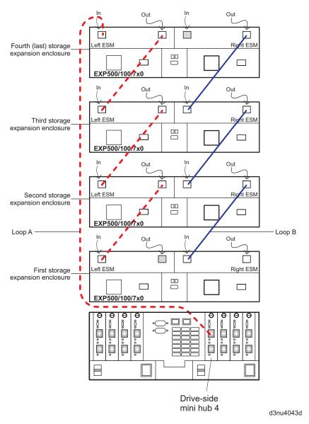
Figure 64. Connecting EXP500, EXP100, EXP700, or EXP710 drive loop A to the DS4500
