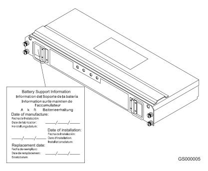
Figure 96. Checking the battery service date
