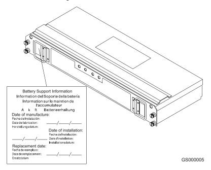
Figure 101. Recording the battery support information
