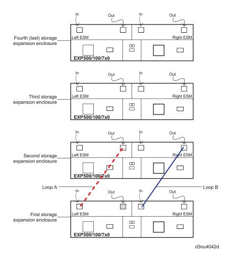
Figure 61. Connecting two EXP500, EXP100, EXP700, or EXP710 storage expansion enclosures into redundant drive loop B
