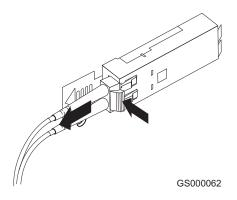
Figure 42. Removing the LC-LC fibre-channel cable
