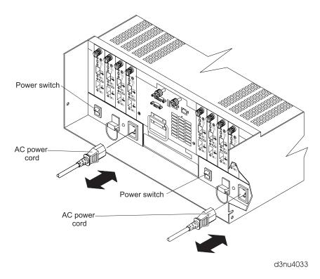
Figure 84. Connecting the power cords
