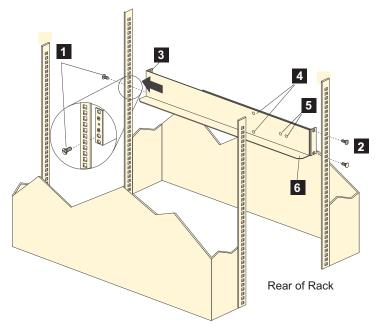
Figure 20. Installing the support rails
