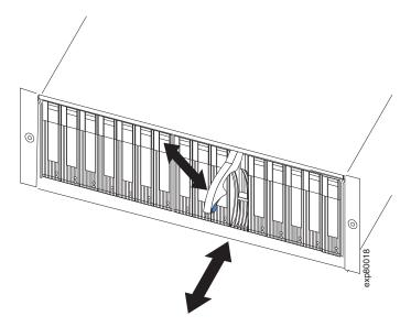
Figure 30. Replacing an E-DDM
