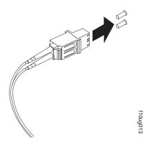
Figure 43. Removing the LC-SC cable adapter protective caps
