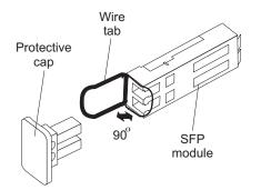
Figure 36. Unlocking the SFP module latch - wire variety
