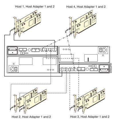
Figure 78. Cabling diagram for four redundant host connections
