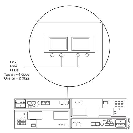
Figure 104. Link rate LEDs
