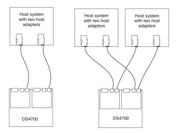
Figure 79. Examples of redundant host direct attached fibre channel configurations
