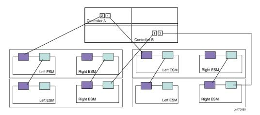
Figure 54. One DS4700 Express and four storage expansion enclosure — Recommended cabling
