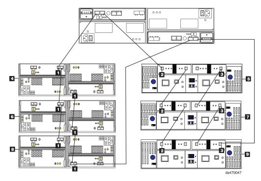
Figure 70. One DS4700 Express and two or more storage expansion enclosures in a mixed environment — Recommended cabling
