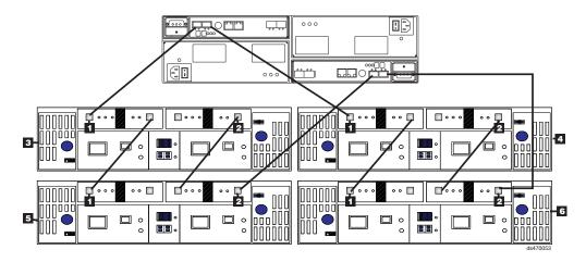
Figure 63. One DS4700 Express and four EXP710 storage expansion enclosures behind a pair of DS4700 drive ports
