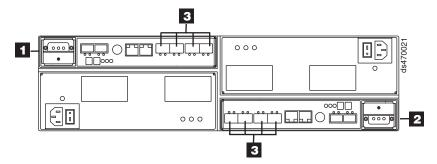
Figure 76. Location of host cables on RAID controllers on model 72 of the DS4700 Express
