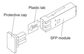
Figure 34. Installing an SFP module into the host port
