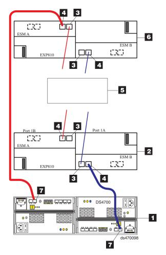
Figure 58. DS4700 Express drive ports connected to EXP810 ESM ports labeled 1B
