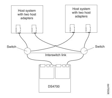
Figure 80. Example of a single SAN fabric configuration
