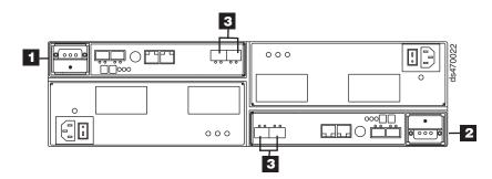
Figure 75. Location of host cables on RAID controllers on model 70 of the DS4700 Express
