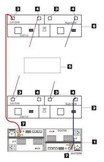
Figure 59. DS4700 Express drive ports connected to EXP710 ESM In and Out ports
