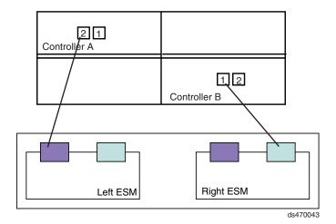
Figure 50. One DS4700 Express and one storage expansion enclosure — Recommended cabling
