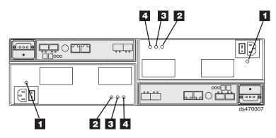
Figure 88. Power supply and fan unit LEDs
