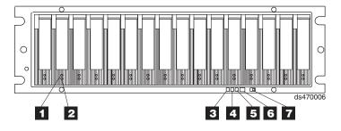
Figure 90. Front LEDs and controls
