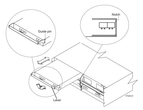
Figure 27. Removing and replacing a controller
