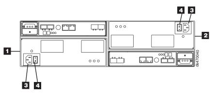
Figure 4. Power supply and fan unit components for DS4700 Express model 70
