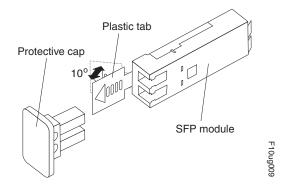
Figure 97. Unlocking the SFP module latch - plastic variety
