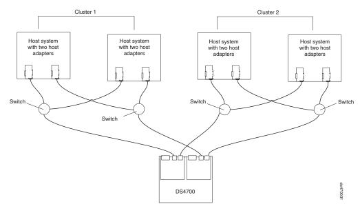
Figure 83. Example of a two-cluster configuration
