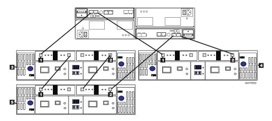
Figure 62. One DS4700 Express and three EXP710 storage expansion enclosures behind a pair of DS4700 drive ports
