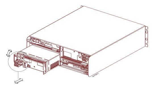
Figure 107. Replacing a DC power supply and fan unit
