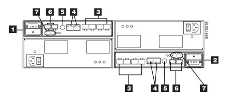
Figure 3. Back view; connectors, switch, ports, enclosure ID on model 72
