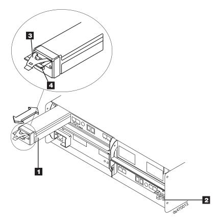
Figure 108. Removing and replacing a battery unit from the controller chassis
