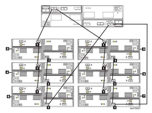
Figure 69. One DS4700 Express and a maximum of six EXP810 storage expansion enclosures behind a pair of DS4700 drive ports
