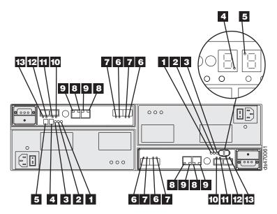
Figure 92. Rear controller LEDs, controls, and connectors - Model 70
