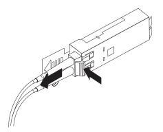
Figure 41. Removing the LC-LC fibre-channel cable
