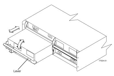
Figure 28. Replacing a power supply and fan unit
