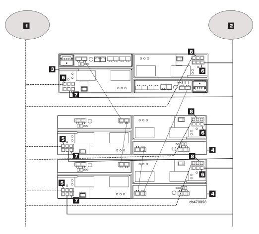
Figure 85. DC power supply and fan unit cabling scheme - dual-level redundancy
