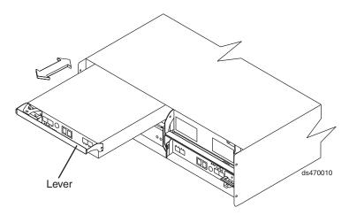
Figure 21. Removing and replacing a controller
