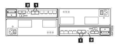
Figure 72. Ethernet and serial port locations on DS4700 Express model 72
