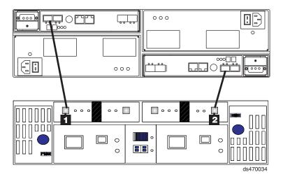
Figure 60. One DS4700 Express and one EXP710 storage expansion enclosure — Recommended cabling
