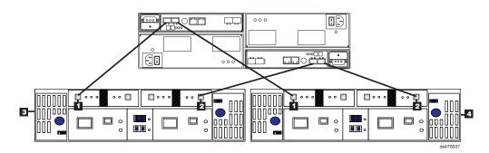
Figure 61. One DS4700 Express and two EXP710 storage expansion enclosures behind a pair of DS4700 drive ports
