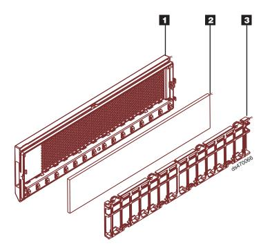
Figure 13. Filter and filter retainer
