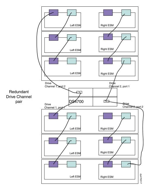
Figure 47. Example of a redundant drive channel pair
