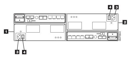
Figure 5. Power supply and fan unit components for DS4700 Express model 72
