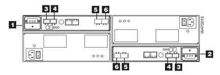
Figure 48. DS4700 Express Storage Subsystem (Model 70) ports and controllers
