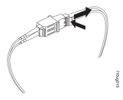
Figure 46. Removing the LC-LC fibre-channel cable from an LC-SC fibre-channel cable adapter
