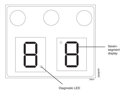
Figure 94. Numeric display LEDs
