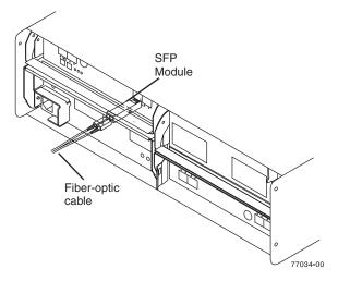
Figure 11. SFP module and fiber optic cable
