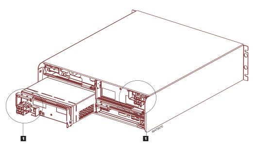
Figure 7. DC power supply and fan unit
