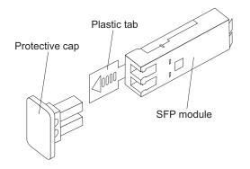
Figure 33. SFP module and protective cap
