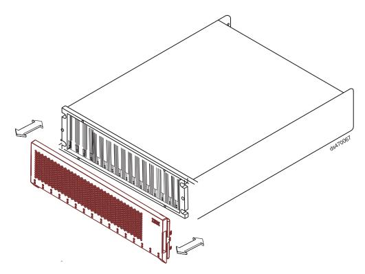
Figure 101. Removing and replacing a bezel
