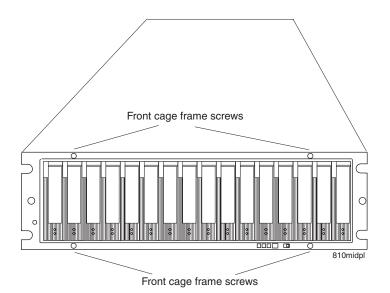
Figure 110. Front cage frame screw locations
