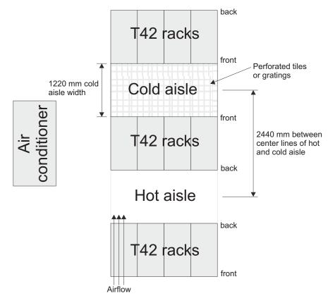
Figure 16. Example of cold aisle/hot aisle rack configuration
