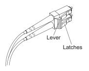
Figure 40. LC-LC fibre-channel cable lever and latches
