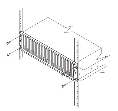
Figure 26. Securing the DS4700 Express to the rack cabinet
