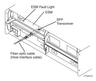
Figure 109. Replacing an SFP module
