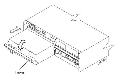
Figure 22. Removing a power supply and fan unit
