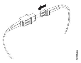
Figure 44. Connecting an LC-LC cable into the LC-SC cable adapter
