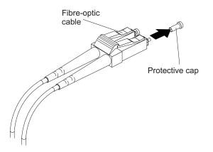
Figure 38. Removing fiber-optic cable protective caps
