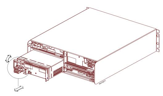
Figure 29. Replacing a DC power supply and fan unit
