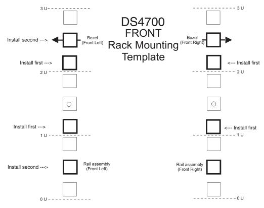
Figure 113. Front rack mounting template
