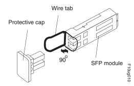
Figure 98. Unlocking the SFP module latch - wire variety
