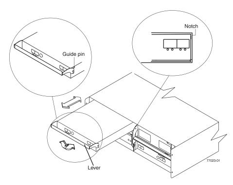
Figure 100. Installing a controller
