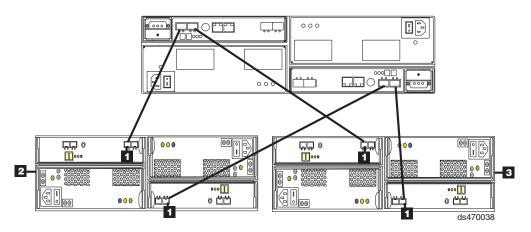
Figure 66. One DS4700 Express and two EXP810 storage expansion enclosures behind a pair of DS4700 drive ports
