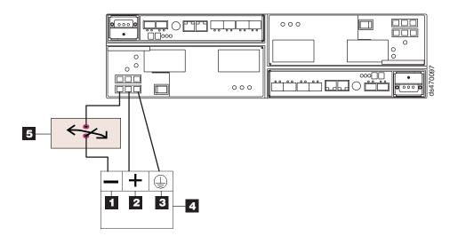
Figure 87. DC wiring from DS4700 Express to disconnect device and DC power source
