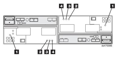
Figure 89. DC power supply and fan unit LEDs
