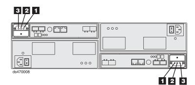
Figure 96. Battery unit LEDs
