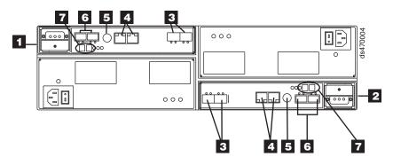
Figure 2. Back view; connectors, switch, ports, enclosure ID on model 70
