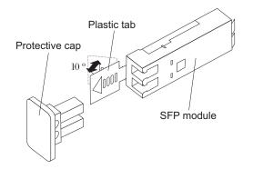
Figure 35. Unlocking the SFP module latch - plastic variety
