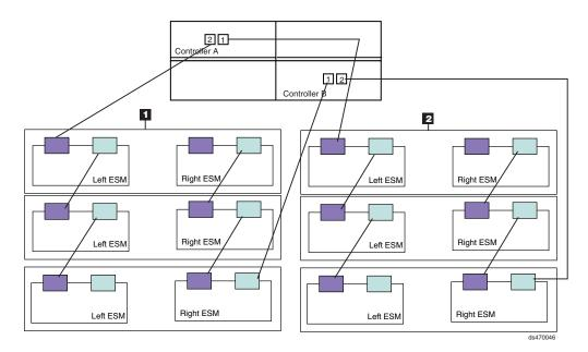
Figure 57. One DS4700 Express and two or more storage expansion enclosures in a mixed environment — Recommended cabling
