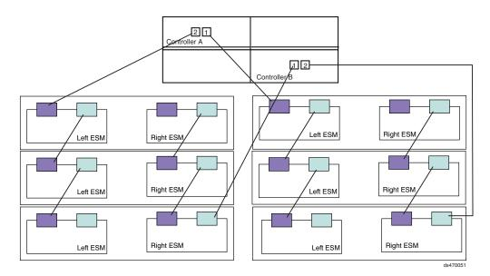
Figure 55. One DS4700 Express and up to six storage expansion enclosure — Recommended cabling
