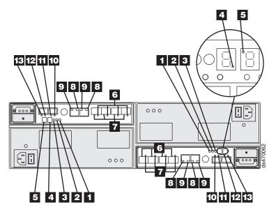
Figure 93. Rear controller LEDs, controls, and connectors - Model 72
