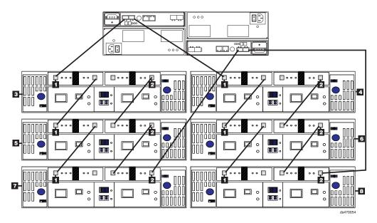
Figure 64. One DS4700 Express and a maximum of six EXP710 storage expansion enclosures behind a pair of DS4700 drive ports
