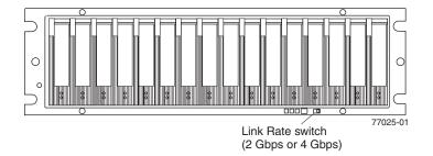
Figure 105. Link rate switch
