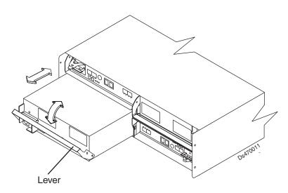
Figure 106. Replacing a power supply and fan unit
