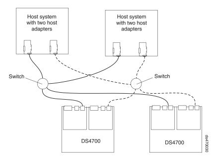
Figure 82. Example of two storage subsystems in a dual SAN environment
