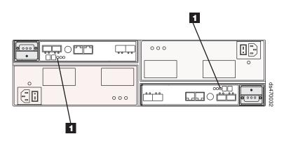
Figure 95. Cache Active LEDs
