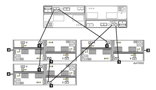
Figure 67. One DS4700 Express and three EXP810 storage expansion enclosures behind a pair of DS4700 drive ports
