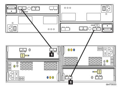
Figure 65. One DS4700 Express and one EXP810 storage expansion enclosure — Recommended cabling
