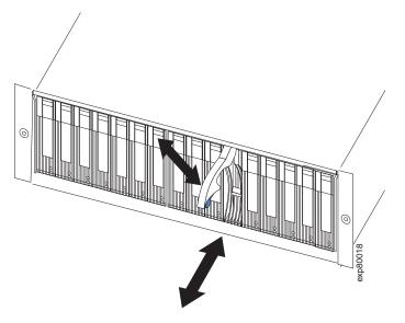
Figure 24. Removing a E-DDM CRU
