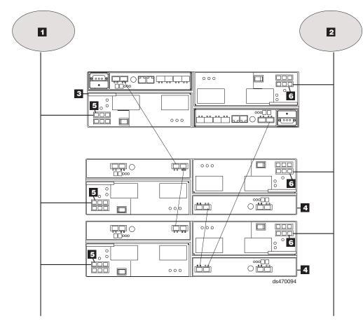
Figure 84. DC power supply and fan unit cabling scheme - single-level redundancy
