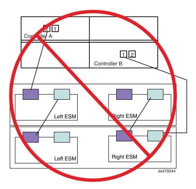
Figure 51. One DS4700 Express and two storage expansion enclosure — Not recommended cabling
