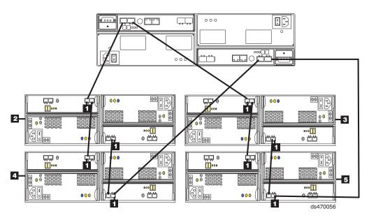
Figure 68. One DS4700 Express and four EXP810 storage expansion enclosures behind a pair of DS4700 drive ports
