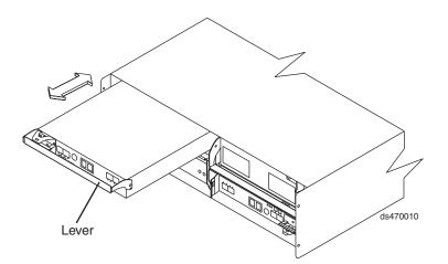
Figure 99. Removing a controller from the DS4700 Express
