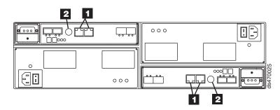
Figure 71. Ethernet and serial port locations on DS4700 Express model 70
