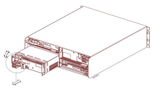
Figure 23. Removing a DC power supply and fan unit
