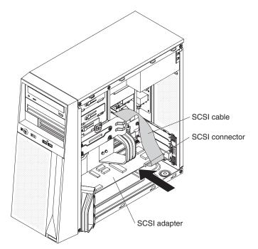
3. Complete the installation of the SCSI adapter (see "Installing an adapter" on page 32).
