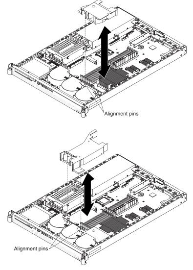
2. Position the internal cables so that they do not interfere with the cover installation.
