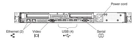
Cable identifiers are printed on the cables that come with the server and optional devices. Use these identifiers to connect the cables to the correct connectors, such as the identifiers in the following examples:
