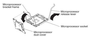
b. Lift the hinged microprocessor bracket frame into the open position.
