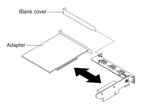
12. Grasp the adapter by its top edge or upper corners; then, align the edge connector on the adapter with the connector on the riser-card assembly. Press the adapter *firmly* into the riser-card assembly connector so that the adapter edge connector seats fully. This secures the adapter in the connector.
