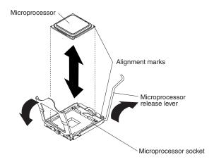
8. Carefully close the release lever to secure the microprocessor in the socket.
