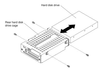
To install a drive in the rear hard disk drive cage, complete the following steps.
