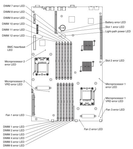
When you press the light path button, the light-path power LED (green) comes on. The light path button enables you to review error indications after the server has been turned off. Press and hold the button, which is behind the operator information panel, to relight the error LEDs that were lit before you removed power from the server. These LEDs and the light-path power LED will remain lit for as long as you press the button, to a maximum of 30 seconds.
