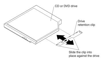
6. Slide the drive into the server until the drive clicks into place.
