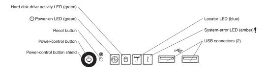
The following controls, LEDs, and connectors are on the operator information panel:
