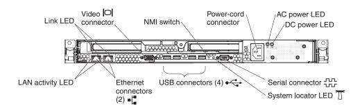
**Link LEDs (Ethernet):** These LEDs are on the dual Ethernet connector. When either LED is lit, it indicates that there is an active link between the server and the network device that is connected to the left or right connector.
