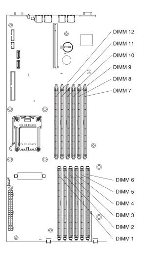
To install a DIMM, complete the following steps.
