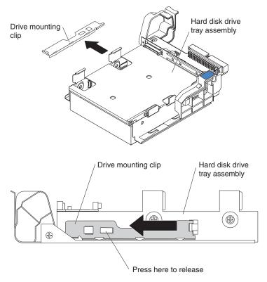
Then, slide the drive mounting clip to attach it to the side of the drive.
