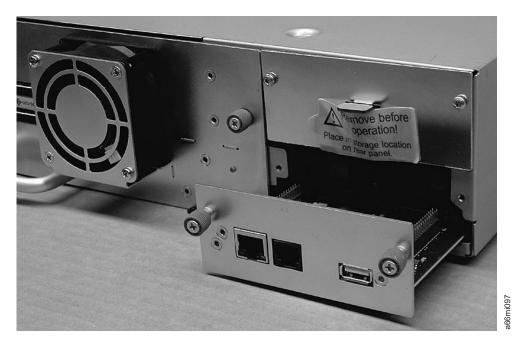
Figure 23. Remove controller card
