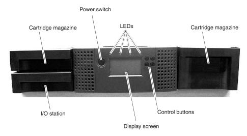
Figure 1. Front panel components
