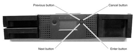
Figure 4. Control panel buttons
