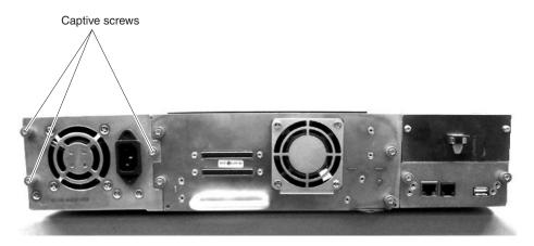
Figure 24. Remove power supply
