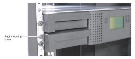
Figure 22. Removing the chassis
