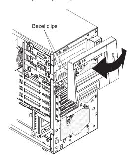
2. Install the lower bezel on the front of the server chassis.
