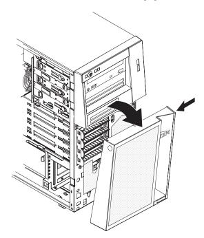
4. Lift the lower bezel to disengage the two bottom tabs from the chassis. Set the lower bezel aside.
