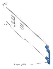
Carefully grasp the adapter by the top edge or upper corners, and align it with the expansion-slot guides; then, press the adapter *firmly* into the expansion slot. Move the adapter directly from the static-protective package to the expansion slot.
