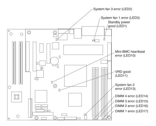
Use the system-board LEDs to diagnose system errors. Each error LED is lit to indicate a problem with a specific component. After a problem is corrected, its LED will not be lit the next time that the server is restarted; if the problem remains, the LED will be lit again. For additional information, see the *Problem Determination and Service Guide* on the IBM *xSeries Documentation* CD.
