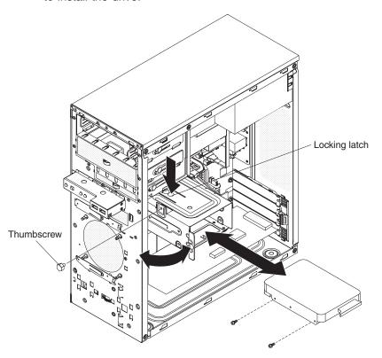
6. Touch the static-protective package that contains the drive to any unpainted metal surface on the server; then, remove the drive from the package and place it on a static-protective surface.
