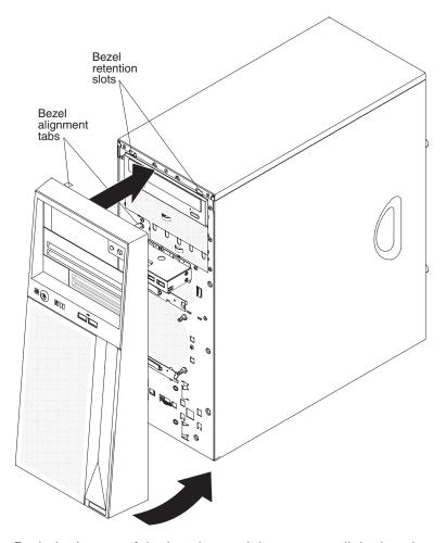
2. Push the bottom of the bezel toward the server until the bezel snaps into place.
