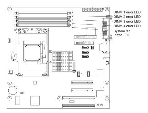
Each error LED is lit to indicate a problem with a specific component. After a problem is corrected, its LED will not be lit the next time the server is restarted; if the problem remains, the LED will be lit again. See the *Problem Determination and Service Guide* on the IBM *System x Documentation* CD for additional information.
