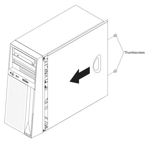
3. Use the two thumbscrews that you removed earlier to secure the cover to the server chassis.
