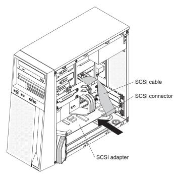
3. Complete the installation of the optional SCSI adapter (see "Installing an adapter" on page 23).
