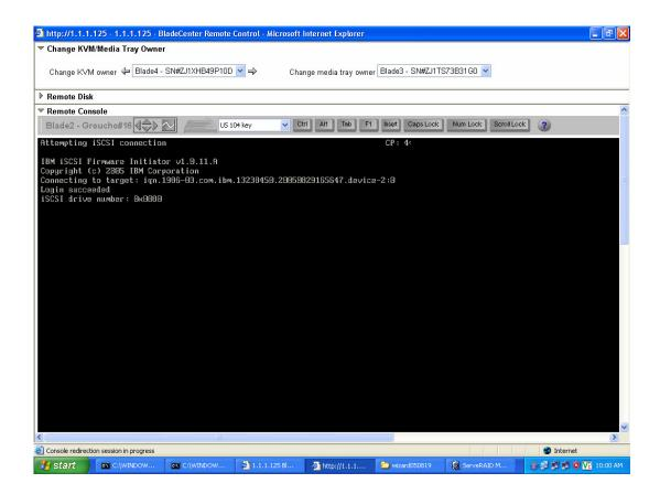
Figure 25: BIOS Panel of a Successful iSCSI Login to an iSCSI Target As the booting process proceeds, additional information is provided. Below is a screen shot of a SUSE boot on a diskless blade
