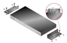
Figure 2.2: Appliance vertical installation
