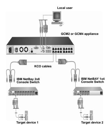
Figure 2.5: Appliance configuration with an earlier-model appliance
