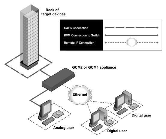
Figure 1.3: Example appliance configuration
