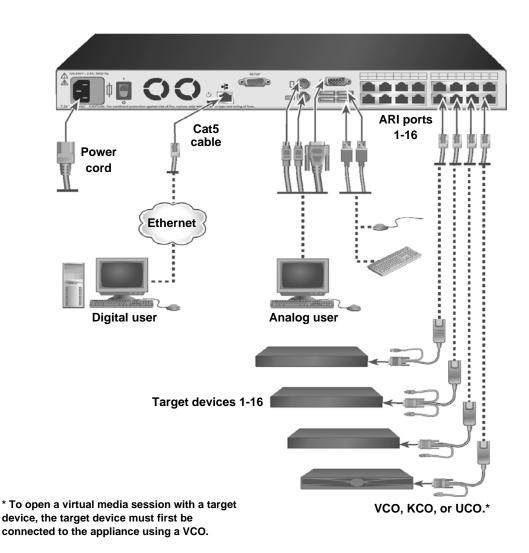
Figure 2.1: Basic appliance configuration
