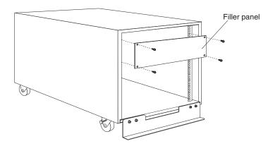
Figure 11. Installing a blank filler panel
