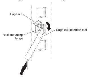
Figure 7. Installing cage nuts with the cage-nut-insertion tool
