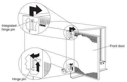
Figure 3. Removing the front door from the rack cabinet
