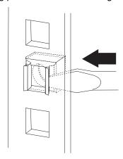
Figure 8. Installing cage nuts with a flat-blade screwdriver
