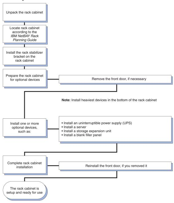
Figure 1. Installing the rack cabinet and devices overview
