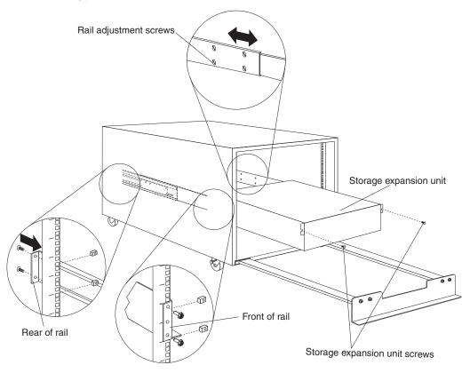
Figure 10. Installing a storage expansion unit
