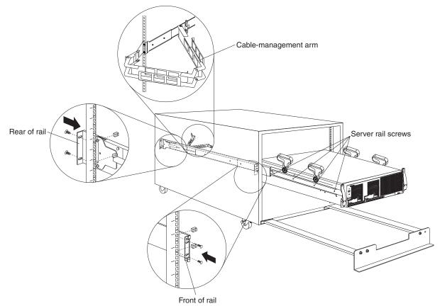
Figure 9. Installing a server
