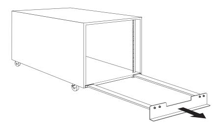
Figure 5. Extending the stabilizer bracket
