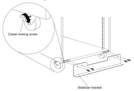
Figure 4. Locking the casters and installing the stabilizer bracket
