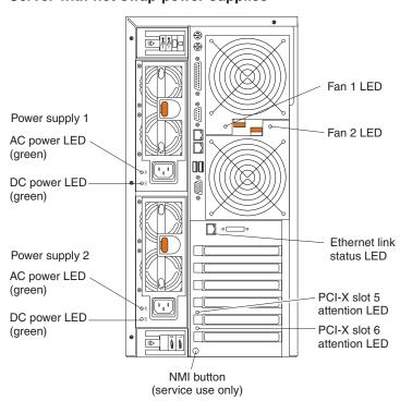
Fans 1 and 2 LEDs: These LEDs provide status information about fans 1 and 2 (the rear fans in connector J25). For additional information, see the "Light path diagnostics" in the Hardware Maintenance Manual and Troubleshooting Guide on the IBM xSeries Documentation CD.
