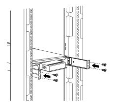
15. Install the screw that attaches the cable-management arm to the left slide-rail bracket; then, tighten all four slide-rail-adjustment screws.
