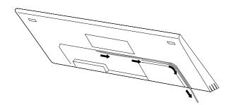
Peel the protective strip from the hook-and-loop-fastener strip inside the keyboard storage area; then, route the keyboard and mouse connectors through the small round opening on the right side of the tray.
