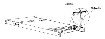
3. Fully extend the tray; then, carefully lift the rear of the flat panel monitor and raise the monitor to the full upright position.
