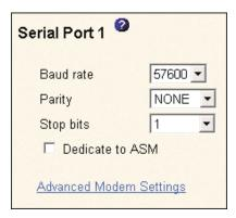
3. In the Baud rate field, select the data transfer rate.
