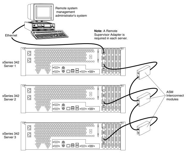
**Note:** The ASM Interconnect module is attached to the RS-485 P-P (peer to peer) port on the back panel of the Remote Supervisor Adapter in each server.
