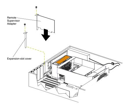
b. Press the adapter *firmly* into the PCI slot.
