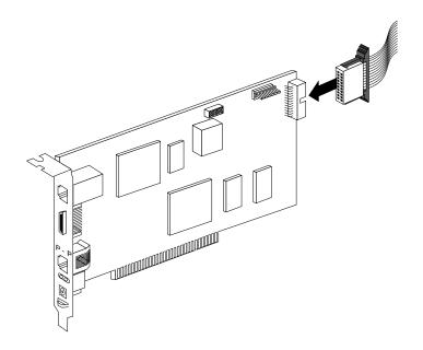
b. Connect the other end of the 20-pin ribbon cable to the system-management connector (J57) on the system board. For the location of the system-management connector, see the illustration in step 8b.
