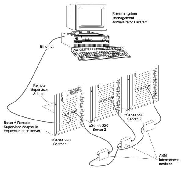
**Note:** The ASM Interconnect module is attached to the RS-485 P-P (peer to peer) port on the back panel of the Remote Supervisor Adapter in each server.
