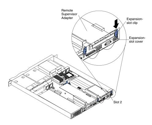
6. Remove the expansion-slot cover from PCI slot 2. Store it in a safe place for future use.
