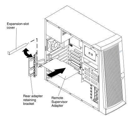
6. Remove the expansion-slot cover from PCI slot 2. Store it in a safe place for future use.
