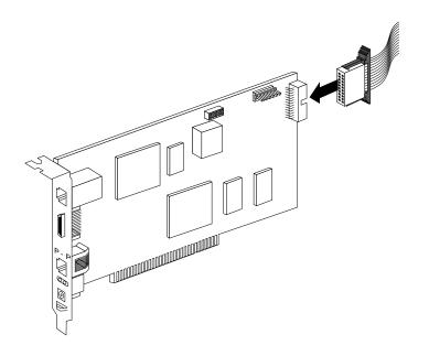
b. Connect the other end of the cable to the system-management connector (J54) on the system board.
