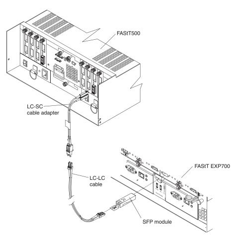
Figure 31. Connecting the FAStT500 to the FAStT EXP700
