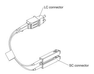
Figure 23. LC-SC Fibre Channel cable adapter
