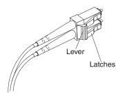
Figure 21. LC-LC Fibre Channel Cable lever and latches
