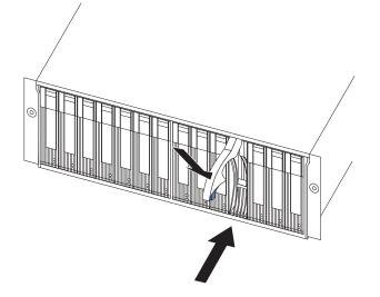
Figure 39. Closing the hot-swap hard disk drive tray handle
