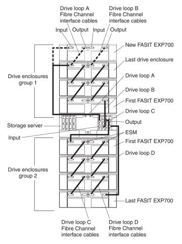
Figure 34. Cabling the FAStT EXP700 to a loop
