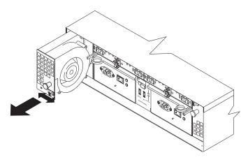
Figure 43. Replacing a hot-swap cooling fan
