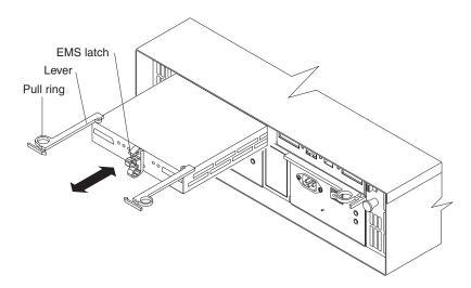
Figure 7. Removing an ESM
