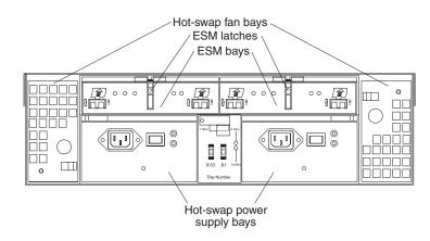
Figure 2. Hot-swap fan, ESM, and power supply bays
