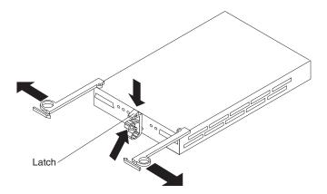
Figure 42. Removing the failed ESM
