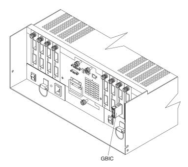
Figure 30. Installing a GBIC in a FAStT500
