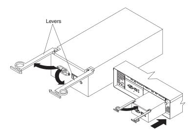
Figure 12. Replacing a power-supply CRU
