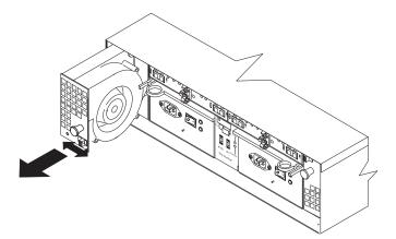
Figure 9. Removing a fan CRU
