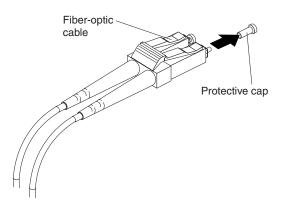
Figure 19. Removing fiber-optic cable protective caps
