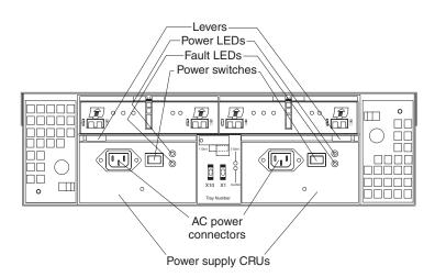
Figure 4. Power-supply controls, indicators, and connectors
