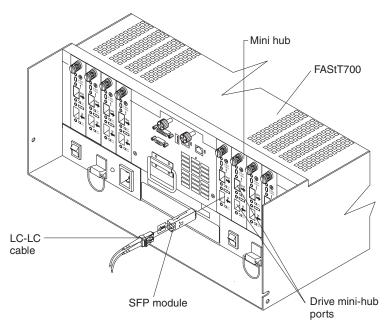
Figure 32. Installing an SFP module and LC-LC cable in a FAStT700
