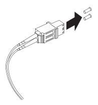
Figure 24. Removing the LC-SC cable adapter protective caps
