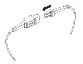
Figure 25. Connecting an LC-LC cable into the LC-SC cable adapter
