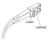
Figure 26. LC-LC Fibre Channel cable lever and latches
