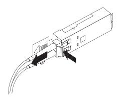
Figure 22. Removing the LC-LC Fibre Channel cable
