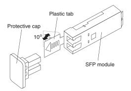
Figure 17. Unlocking the SFP module latch
