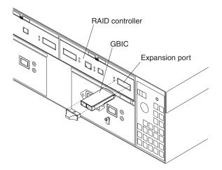
Figure 28. Installing a GBIC in a FAStT200
