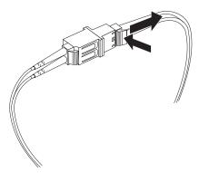
Figure 27. Removing the LC-LC Fibre Channel cable from an LC-SC Fibre Channel cable adapter
