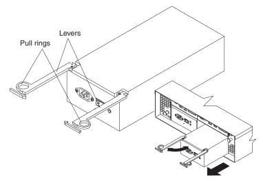
Figure 8. Removing a power supply CRU
