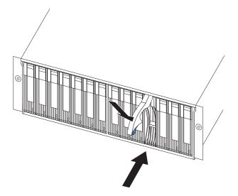
Figure 14. Replacing hot-swap hard disk drives
