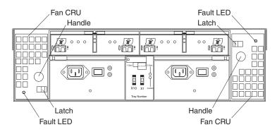
Figure 5. Fan controls and indicators
