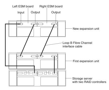
Figure 35. FAStT EXP700 redundant loop configuration
