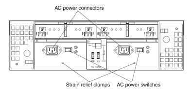
Figure 41. Connecting the power supply
