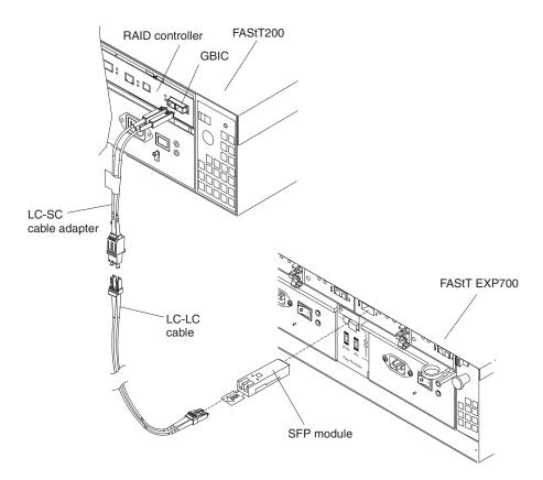
Figure 29. Connecting the FAStT200 to the FAStT EXP700
