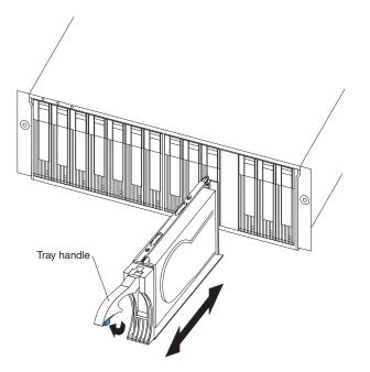
Figure 10. Removing drive CRUs
