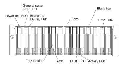
Figure 3. Front controls and indicators
