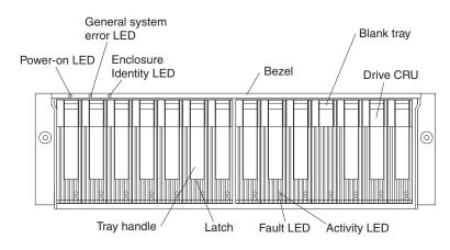
Figure 36. Hot-swap hard disk drive LEDs
