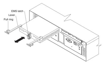
Figure 11. Replacing an ESM
