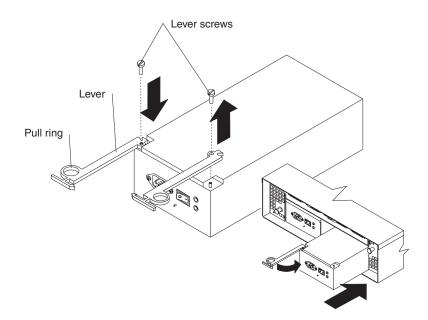
Figure 40. Moving the power-supply lever and replacing the failed hot-swap power supply
