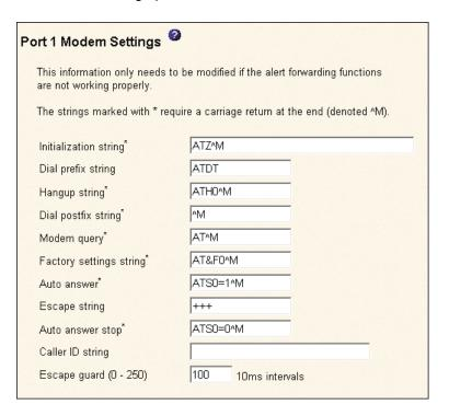
Set these values only if the alert forwarding functions are not working properly. The strings marked with an asterisk (\*) require a carriage return (^M) to be manually entered at the end of the field value.
