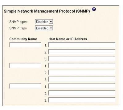
4. Enable the SNMP agent and SNMP traps fields.
