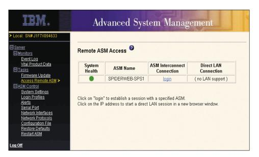
3. In the ASM Interconnect Connection column for the entry that matches the ASM processor of the server that you want to monitor, click **login**.
