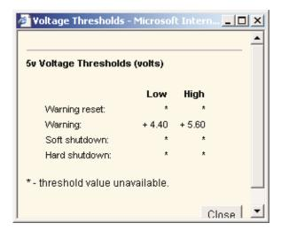
The Voltage Thresholds window displays the voltage ranges at which the ASM processor reacts. These levels are select on the remote server and cannot be changed.
