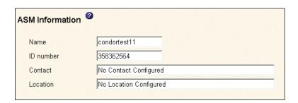
3. In the Name field, type the name of the Remote Supervisor Adapter or the ASM processor. The name is included with e-mail, SNMP, and alphanumeric pager alert notifications to identify the source of the alert.
