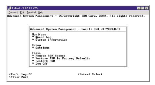
**Note:** Press the Up Arrow and Down Arrow keys to navigate this screen. Press Esc to exit to the Advanced System Management window; if you press Esc at the Advanced System Management window, you log off from your session. Press F3 to exit the window you are viewing.
