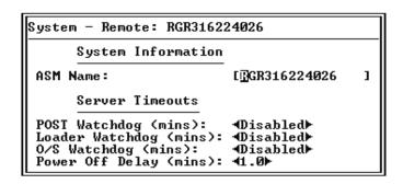
5. In the ASM Name field, type the name of the Remote Supervisor Adapter.
