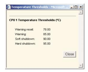
The Temperature Thresholds window displays the temperature levels at which the ASM processor reacts. These levels are select on the remote server and cannot be changed.
