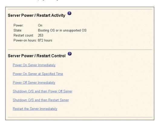
State The State field shows the state of the system when this Web page was generated. Possible states include:
