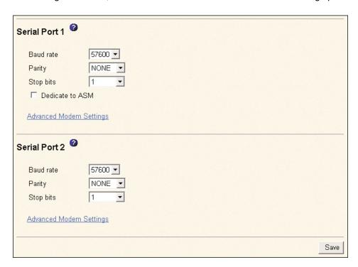
**Note:** Only Serial Port 1 appears on the Serial Port page when you are logged into the Remote Supervisor Adapter.
