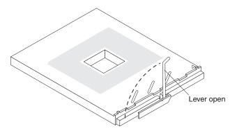
Figure 30. Opening the microprocessor-release lever
