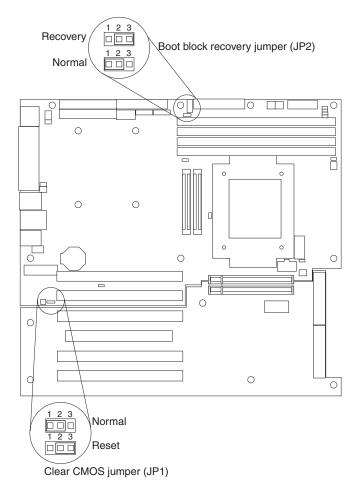
Figure 8. Location of recovery jumpers on system board
