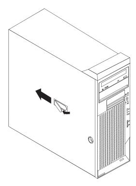
Figure 10. Removing the side cover
