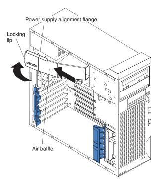
Figure 40. Removing the air baffle
