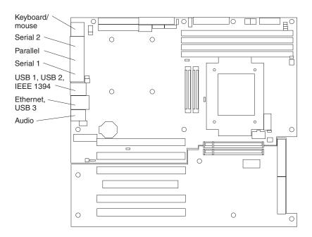
Figure 4. System-board external connectors
