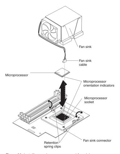
Figure 32. Installing a microprocessor and fan sink
