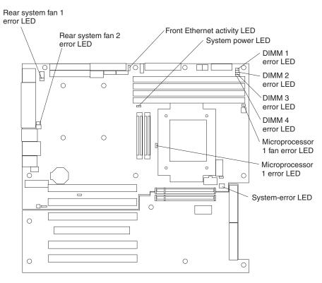
Figure 5. System-board LEDs
