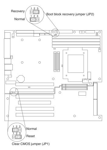
Figure 6. System-board jumpers
