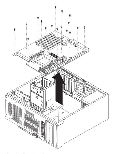
Figure 43. System board removal
