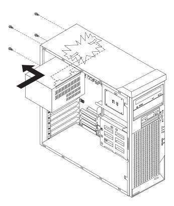
Figure 42. Replacing the power supply
