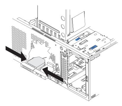
Figure 39. Front USB connector assembly replacement
