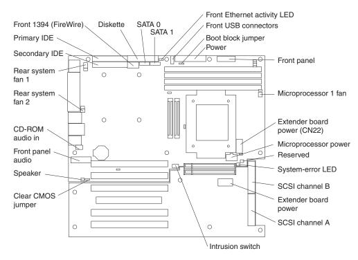
Figure 3. System-board internal connectors
