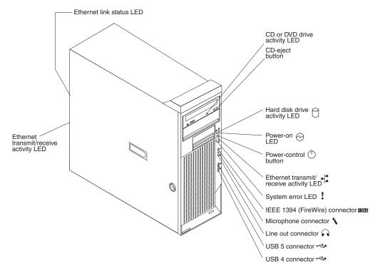
Figure 1. Controls, LEDs, and indicators
