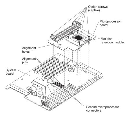
Figure 34. Removing the microprocessor board
