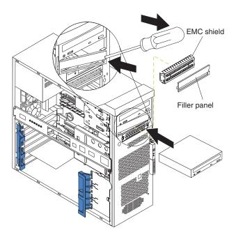
Figure 18. Installing a drive in bay 3
