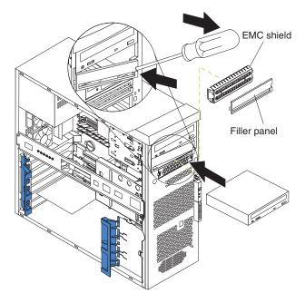
Figure 16. Preparing to install a drive in bay 2
