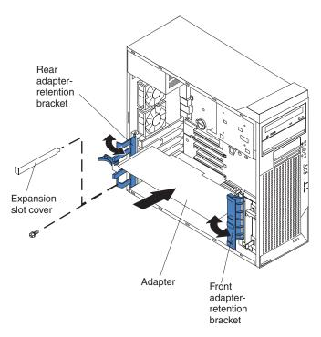
Figure 13. Adapter placement
