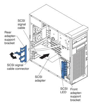
Figure 14. SCSI signal cable placement
