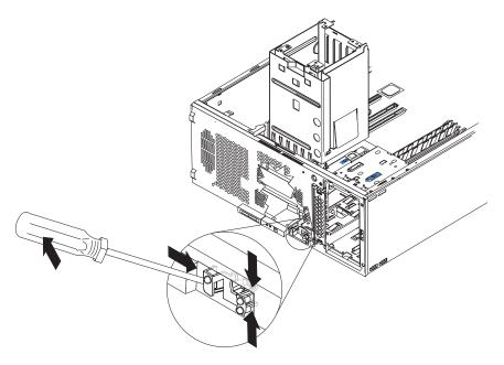
Figure 37. Control panel assembly replacement
