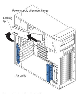
Figure 27. Installing the baffle
