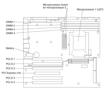
Figure 2. System-board option connectors
