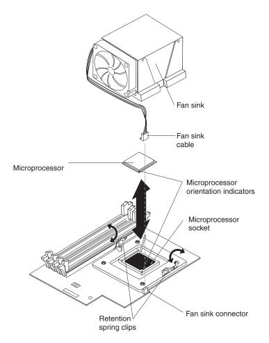
Figure 28. Connector locations on microprocessor board
