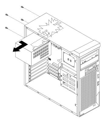
Figure 41. Removing the power supply
