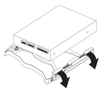
Figure 20. Attaching the drive to the drive tray
