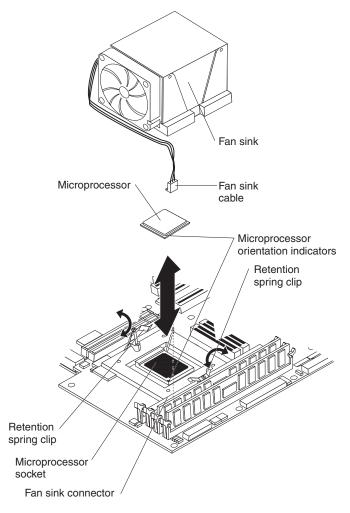
Figure 26. Installing microprocessor 1 and fan sink
