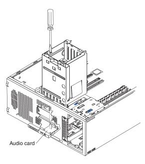
Figure 38. Audio card/FireWire assembly replacement
