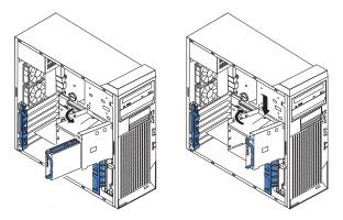
Figure 19. Rotating the drive cage
