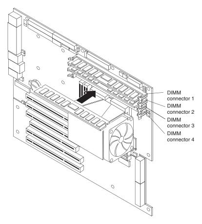
Figure 21. Installation of DIMMs 1-4
