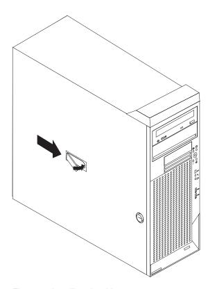
Figure 11. Installing the side cover
