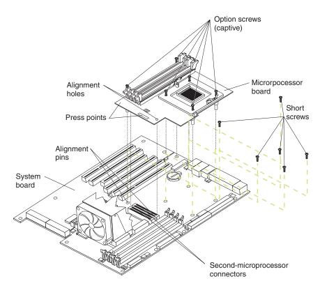
Figure 31. Installing the microprocessor board
