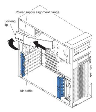
Figure 33. Installing the baffle
