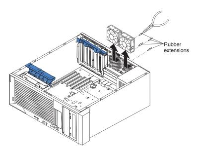
Figure 36. Fan assembly replacement
