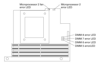
Figure 7. Microprocessor-board diagnostic LEDs
