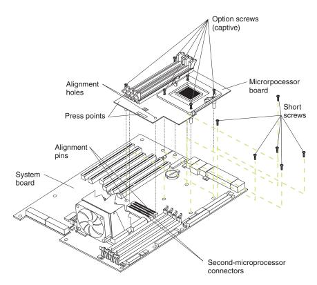
Figure 29. Location of screws on microprocessor board
