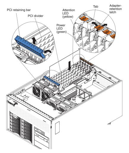
4. See the documentation that comes with the adapter for instructions for setting jumpers or switches and for cabling.
