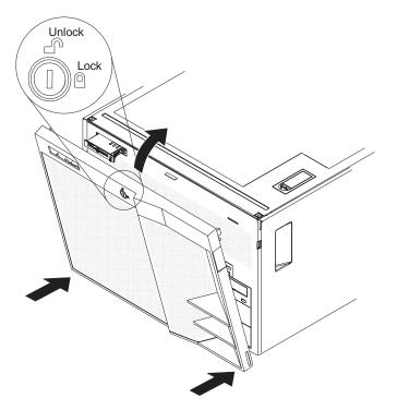
1. Insert the two tabs on the bottom of the front cover into the matching holes on the bezel.
