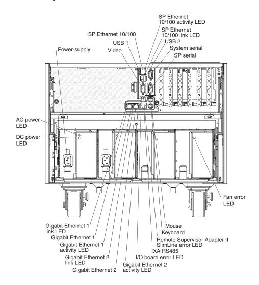
The following illustration shows the connectors and LEDs on the rear of the server.
