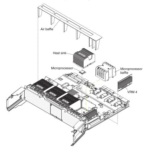
Remove the microprocessor baffle from a microprocessor socket and store it for future use. If you remove a microprocessor you must install a microprocessor baffle to prevent the server from overheating.
