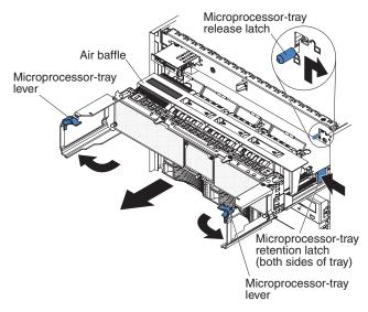
b. Open the microprocessor-tray levers.
