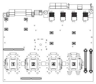
To install an additional microprocessor, complete the following steps:
