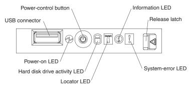
The following controls, connectors, and LEDs are on the operator information panel:
