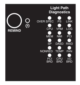
Look at the system service label on the top of the server, which gives an overview of internal components that correspond to the LEDs on the light path diagnostics panel. This information and the information in "Light path diagnostics panel" can often provide enough information to correct the error.
