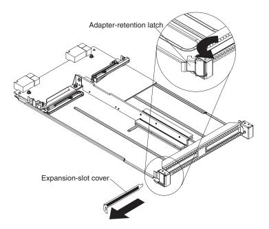
5. Align the PCI adapter with the slot and press the adapter into position as shown in the following illustration. As you install the adapter, apply counter-pressure to the midplane to help prevent any flexing or warping of the midplane.
