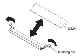
To install a DIMM, complete the following steps:
