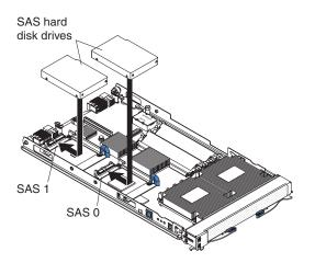
**Note:** Do not install a SAS hard disk drive in SAS connector 1 (J501) if you intend to also install an optional standard-form-factor expansion card. The standard-form-factor expansion card occupies the same area as the second hard disk drive.
