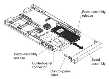
To remove the blade server bezel assembly, complete the following steps:
