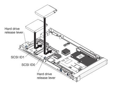
**Note:** Do not install a SCSI hard disk drive in SCSI connector 1 (SCSI ID 1) if you intend to also install an optional standard-form-factor expansion card. The standard-form-factor expansion card occupies the same area as the second hard disk drive.
