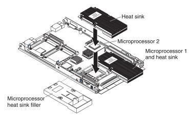
To install an additional microprocessor, complete the following steps:
