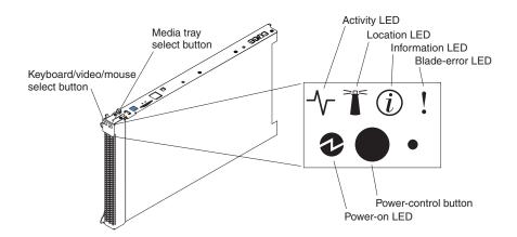
Keyboard/video/mouse (KVM) select button: Press this button to associate the shared BladeCenter unit keyboard port, video port, and mouse port with the blade server. The LED on this button flashes while the request is being processed and then is lit when the ownership of the keyboard, video, and mouse has been transferred to the blade server. It can take approximately 20 seconds to switch the keyboard, video, and mouse control from one blade server to another.
