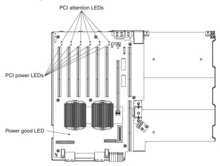
The following illustration shows the LEDs on the PCI-X board.
