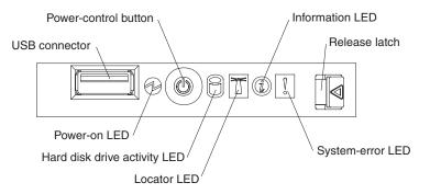
The following controls, connectors, and LEDs are on the operator information panel:
