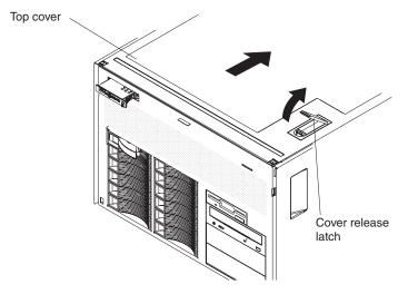
5. Lift the cover-release latch. The cover slides to the rear approximately 13 mm (0.5 inch). Lift the top cover off the server.
