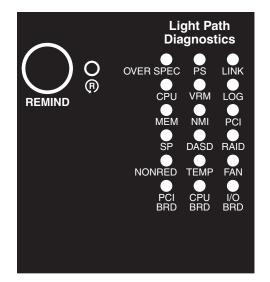
Look at the system service label on the top of the server, which gives an overview of internal components that correspond to the LEDs on the light path diagnostics panel. This information and the information in "Light path diagnostic LEDs" on page 64 can often provide enough information to correct the error.
