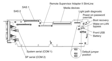
While the server is turned off, move the power-on password jumper from pins 1 and 2 to pins 2 and 3. You can then start the Configuration/Setup Utility program and reset the power-on password. After you reset the password, turn off the server again and move the jumper back to pins 1 and 2.
