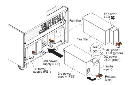
The following table describes the problems that are indicated by various combinations of the power-supply LEDs and the power-on LED on the operator information panel. The table also provides suggested actions to correct the detected problems.
