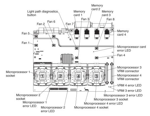
The following illustration shows the connectors and LEDs on the microprocessor board.
