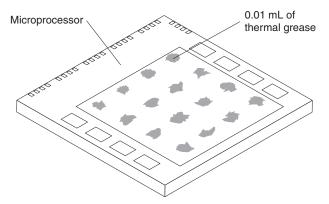
5. Use the thermal-grease syringe to place 16 uniformly spaced dots of 0.01 mL each on the top of the microprocessor.
