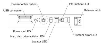
2. To view the light path diagnostics panel, press the release latch on the front of the operator information panel to the left; then, slide it forward. This reveals the light path diagnostics panel. Lit LEDs on this panel indicate the type of error that has occurred.
