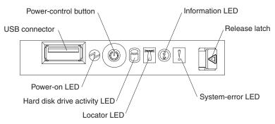
When the information LED on the operator information panel is lit, it indicates that there is a suboptimal condition in the server and that light path diagnostics will light an additional LED to help isolate the condition. If the LOG LED on the light path diagnostics panel is lit, information about the condition is available in the baseboard management controller (BMC) log or in the system-event log. The condition might be that the BMC log is full or almost full.
