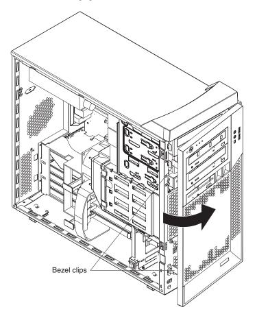
For instructions for replacing the bezel, see "Replacing the bezel" on page 50.
