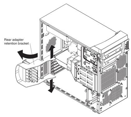
To replace the rear adapter retainer, reverse the steps.
