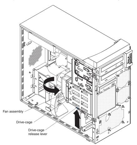
7. Grasp the fan latch on the fan assembly that is over the drive cage and pull it outward to disengage it from the drive cage and rotate it to the side.
