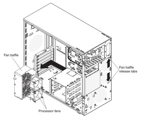
6. Squeeze the fan baffle release tabs so that they release from the notches in the chassis.
