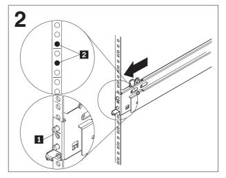
Align the slide rail with the front mounting flange by aligning the score mark on the slide rail with the score mark on the rail between the upper and lower U. Push outward on the slide-rail latch to close the latch and secure the slide rail. Do the same for the other front slide rail. Align the slide rail with the rear mounting flange. The slide rail occupies the full height of the server. Close the latches to secure the rear of both slide rails.
