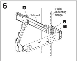
Lift the locking levers **1** on the slide rails and slide the server into the rack until it extends approximately 4 inches from the rack.
