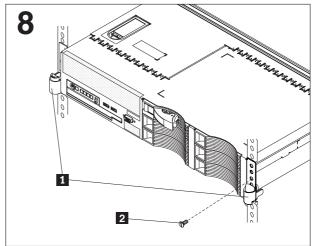
Attach the power cords and other cables to the rear of the server (including keyboard, monitor, and mouse cables, if required). Route the cables and power cords through the slots in the cable-restraint brackets 1. Secure the cable-restraint bracket to the slide rail.
