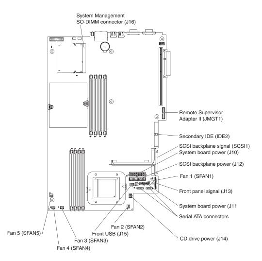
The following illustration shows the internal connectors on the system board.
