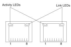
Connect Category 3, 4, or 5 unshielded twisted-pair cables to these connectors. The 100BASE-TX and 1000BASE-T Fast Ethernet standards require Category 5 or higher cabling.
