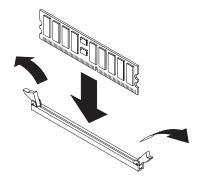
7. Insert the DIMM into the connector by aligning the edges of the DIMM with the slots at the ends of the DIMM connector. Firmly press the DIMM straight down
