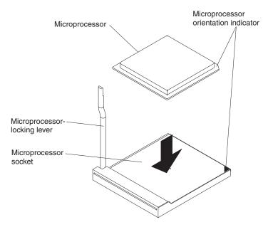
6. Close the microprocessor-locking lever to secure the microprocessor.
