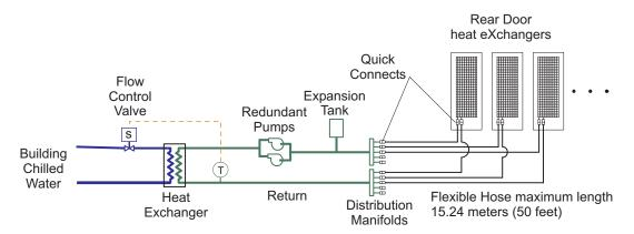
Figure 3. Coolant distribution using a fabricated facilities solution
