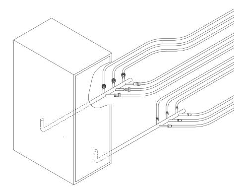
*Figure 5. Typical central distribution manifold layout in a central location* Figure 6 on page 9 shows another layout for multiple water circuits.
