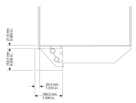
Figure 9. Raised floor hose management example 1; tile cut out size and position
