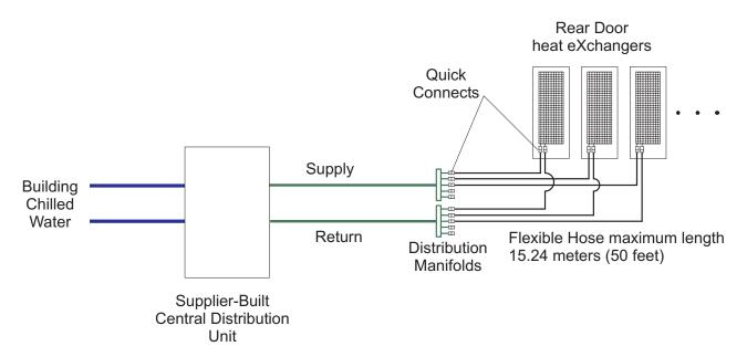
Figure 4. Coolant distribution using off-the-shelf supplier solutions
