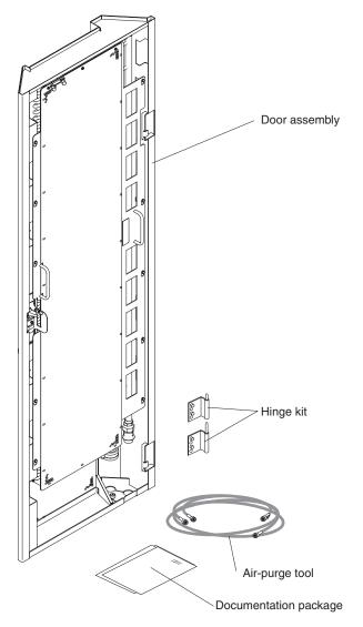
Figure 1. Components of the heat exchanger option kit
