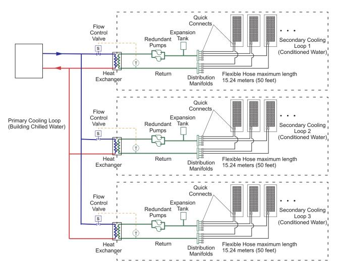
Figure 2. Primary and secondary cooling loops
