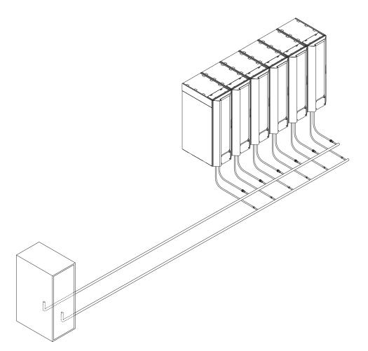
Figure 7. Typical extended manifold (located along aisles between racks)
