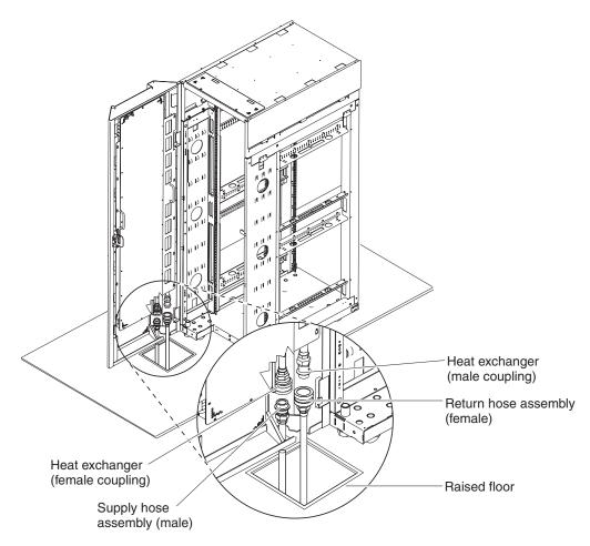
Figure 8. Raised floor hose management example 1; hose exit through floor tile at the door hinge
