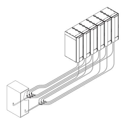
Figure 6. Typical central manifold (located at a central location for multiple water circuits)
