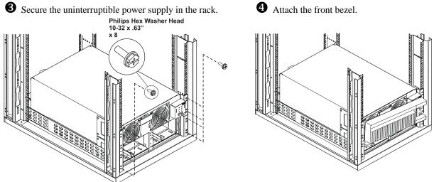
Installing and Connecting the Batteries and Attaching the Front Battery Bezel
