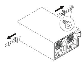
**3** Reinstall the remaining three battery modules.
