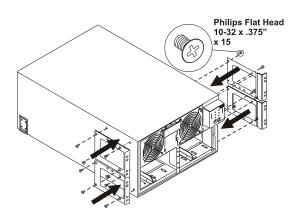
**2** Install the rails per the rail installation diagram in the Rail Kit. Install the cage-nuts (or clip-nuts) and mount the uninterruptible power supply at the bottom of the rack.
