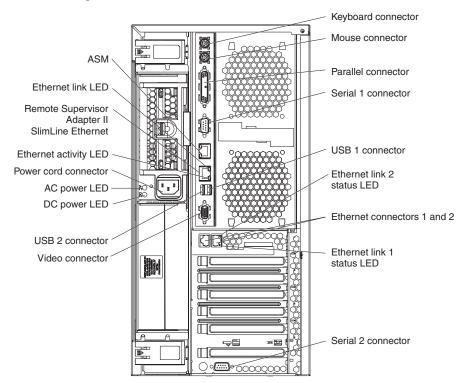
**Keyboard connector:** Connect a PS/2<sup>®</sup> keyboard to this connector.
