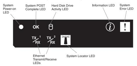
The following LEDs are on the operator information panel:
