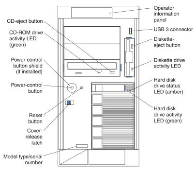
**Operator information panel:** This panel contains LEDs. The following illustration shows the LEDs on the operator information panel.
