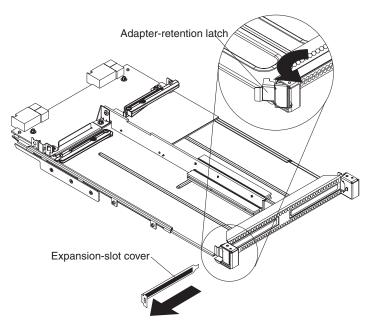
4. Align the PCI adapter with the slot and press the adapter into position as shown in the following illustration. As you install the adapter, apply counter-pressure to the midplane to help prevent any flexing or warping of the midplane.
