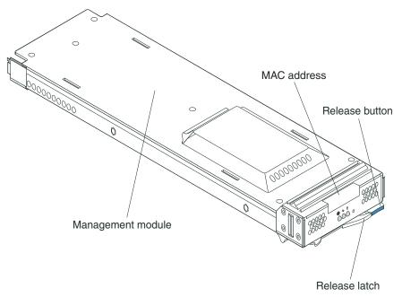
The management module functions as a service processor for the multiple blade servers. The management module configures the BladeCenter T unit and modules, configuring information such as switch module IP addresses. The management module also performs USB-to-PS/2 conversions for the system keyboard and mouse and can send the VGA signal stream to a remote console for viewing. See "Management module controls and indicators" on page 52 for information about the controls and indicators.
