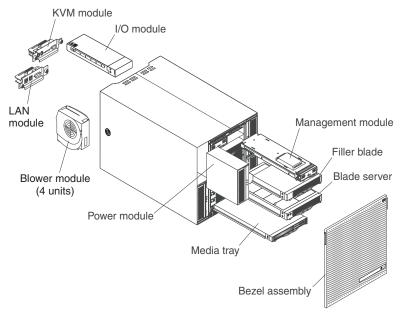
**Attention:** To maintain proper system cooling, each module bay must contain either a module or a filler module; each blade bay must contain either a blade server or a filler blade.
