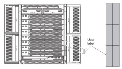
**Important:** Do not place the label on the blade server itself or in any way block the ventilation holes on the blade server.
