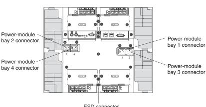
power connector 1 supplies power to power module 1, and so on.)
