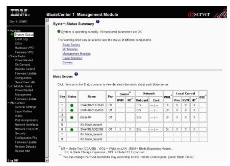
**Note:** The upper left corner of the management and configuration window shows the location and identity of the active management module.
