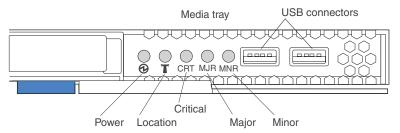
The system-status panel on the front of the BladeCenter T system has five system-status LEDs and two USB connectors.
