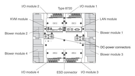
See Chapter 4, "BladeCenter T components, controls, and LEDs," on page 51 for details about the components and indicators.
