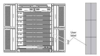
**Important:** Do not place the label on the blade server or in any way block the ventilation holes on the blade server.
