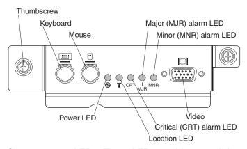
**System-status LEDs:** These LEDs provide status information for the BladeCenter T unit.
