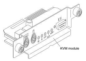
Use the instructions in this section to remove or install the KVM module from the rear of the BladeCenter T unit. The KVM module is held in place by captive thumbscrews. You can use either your fingers or a screwdriver to install or remove the KVM module. If you use a screwdriver, make sure that you do not overtighten the thumbscrews.
