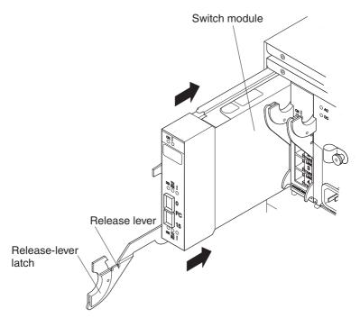
**9**. Push the release lever on the front of the switch module to the closed position. After you insert and lock the switch module, it is turned on, and a POST occurs to verify that the switch module is operating correctly.
