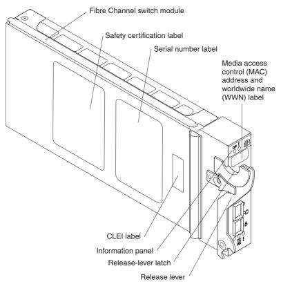
For more information about the components of the information panel, see Chapter 3, "Information panel LEDs and external Fibre Channel ports," on page 21. For more information about the MAC address, see the *Brocade Fabric OS Procedures Guide* on the IBM *Brocade Enterprise/Entry SAN Switch Module for IBM @server BladeCenter Documentation* CD.
