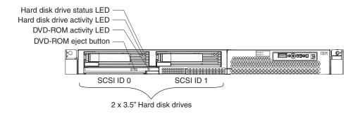
The following illustration shows the front view of an IBM xSeries 336 server with a 3.5-inch SATA simple swap hard disk drive configuration, with the optional DVD-ROM drive.
