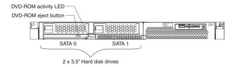
The following information gives details about the previously mentioned controls, LEDs, and connectors on the front of the server. The location of these items vary, depending on the hardware configuration you have.
