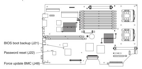
**Attention:** Before changing any switch settings or moving any jumpers, turn off the server; then, disconnect all power cords and external cables. See the safety information beginning on page v. Do not change settings or move jumpers on any system-board switch or jumper blocks that are not shown in this document.
