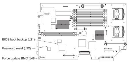
To force the server to start from the backup copy, turn off the server; then, place the J21 jumper in the backup position (pins 2 and 3).
