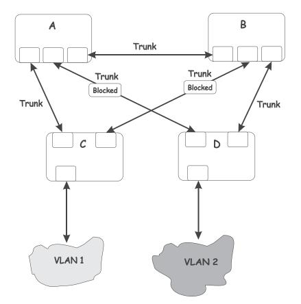
This is a common network design. Through trunks, bridges C and D have redundant links to backbone bridges A and B. Trunks, by default, carry all the VLAN traffic from VLAN 1 and VLAN 2. Therefore, bridge C is not only receiving traffic for VLAN 1, but also unnecessary broadcast and multicast traffic for VLAN 2. Bridge C is also discarding one port for VLAN 2. Thus, there are three redundant paths between bridges A and B, and two blocked ports per VLAN. This increases the chance of a data loop.
