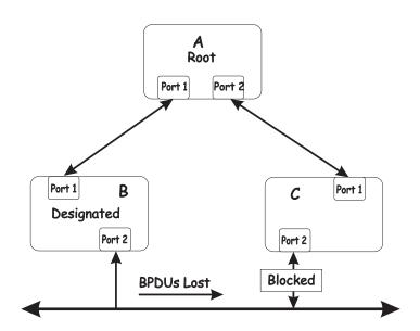
In this example, port 2 on bridge B can receive but not transmit packets. Port 2 on bridge C should be in the discarding state, but since it can no longer receive BPDUs from port 2 on bridge B, it will change to the forwarding state. If the failure exists at boot time, STP will not converge on a stable topology and restarting the bridges will have no effect.
