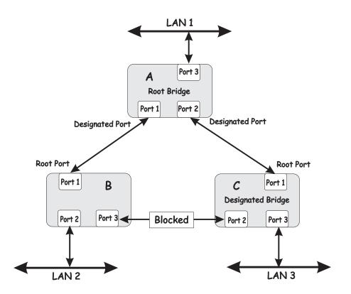
The bridge with the lowest bridge ID (bridge A) was elected the root bridge, and the ports were selected to give a high port cost between bridges B and C.
