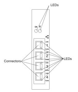
The switch module contains the following internal and external connectors:
