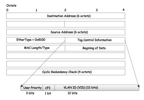
The **EtherType** and **VLAN ID** are inserted after the MAC source address, but before the original **EtherType/Length** or **Logical Link Control**. Because the packet is now longer than it was originally, the cyclic redundancy check (CRC) must be recalculated.
