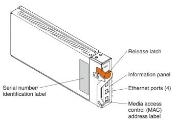
The Ethernet switch-module MAC address can be displayed using the Inventory Information panel on page 64, or by using the CLI command **show inventory**.
