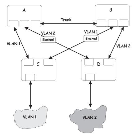
In this example, the VLAN definitions are extended to bridges A and B. This gives only a single blocked port per VLAN and enables the removal of all redundant links by removing bridge A or B from the network.
