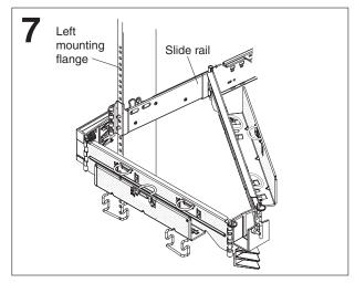
Repeat the previous procedure to attach the cable-management assembly to the left slide rail.
