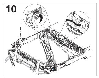
Secure the cables across the rear of the server. Pull the server out of the rack; then, pull the SMP Expansion cables taut from the rear of the server and tighten the retaining straps.
