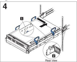
Carefully slide the server along the slide rails approximately one inch toward the rack to lock the server on the slide rails.
