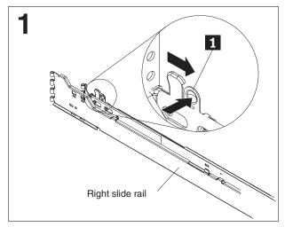
Push outward on the slide-rail latch **1**; then, pull the latch back to open the slide rail. The latch will catch to stay open. Open the other end of the slide rail; then, do the same for the other slide rail. **Note:** The slide rails are marked "Left" and "Right".
