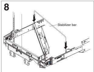
Attach the free end of the cable-management assembly to the slide rail with one end of the stabilizing bar. Attach the other side of the stabilizing bar to the right slide rail.
