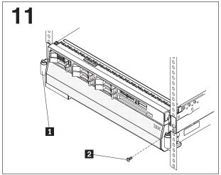
Slide the server into the rack cabinet until the release latches **1** lock into place. To slide the server out of the rack, press on the release latches. **Note:** Insert the optional M6 screws **2** in both sides of the front and rear of the server when moving the rack cabinet, or if you install the rack cabinet in a vibration-prone area.
