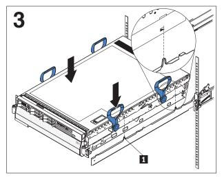
Extend the slide rails fully from the rack until the slide rails lock. Align the tabs on the slide rails **1** with the matching inserts on the server and lower the server onto the slide rails.
