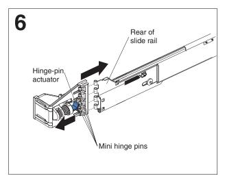
Pull back on the blue hinge-pin actuator on the ramp assembly and place the mini hinge pins of the ramp assembly into the matching hinges of the right slide rail. Push the hinge-pin actuator forward to securely engage the hinge pins.
