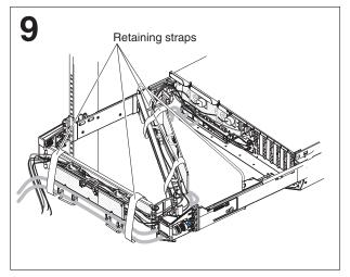
Route the SMP Expansion cables through the wire-form clips.
