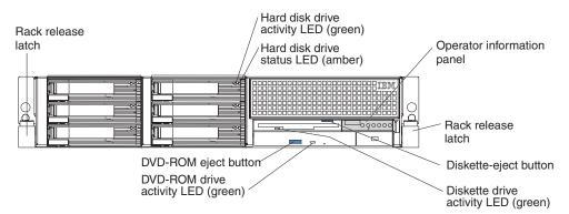
Rack release latches: Press these latches to release the server from the rack.
