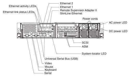
**Ethernet link status LEDs:** When these LEDs are lit, they indicate that there is an active link connection on the 10BASE-T, 100BASE-TX, or 1000BASE-TX interface for the Ethernet port.
