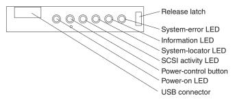
The following controls, LEDs, and connectors are on the operator information panel:
