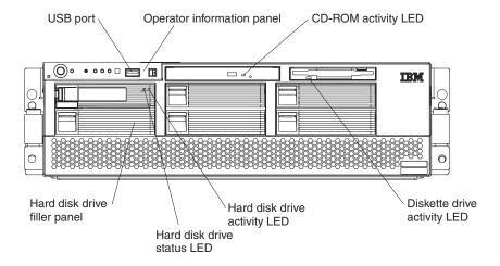
**Operator information panel:** This panel contains controls, indicators, and a USB port. Swing it open to see the light path diagnostics LEDs on the side surface. See "Operator information panel" on page 11 for details.
