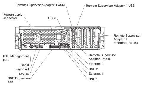
**Power supply connector:** Connect one end of the power-supply power cord to this connector and connect the other end into an ac power source. The server comes with one or two hot-swap power supplies, depending on the server model. If your server comes with one hot-swap power supply, you can add a second hot-swap power supply to obtain full power redundancy. Connect the power supplies to separate ac power circuits for power redundancy.
