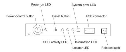
**Power-control button:** Press this button to turn the server on and off manually. A power-control-button shield comes with your server. You can install this disk-shaped shield to prevent the server from being turned off accidentally.
